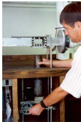
Fig. 2 - Photographs of the Erosion Function Apparatus (a) General View (b) Close-up of the Test Section
