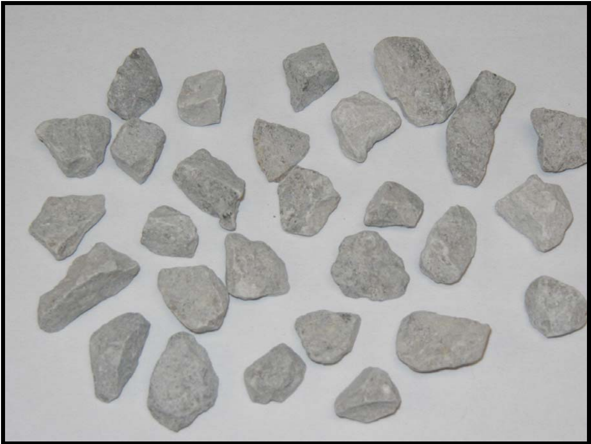
Figure D2. Martin Marietta Limestone Aggregate Particles, Texas Passing 25 mm and Retained on 12.5 mm Sieve.
