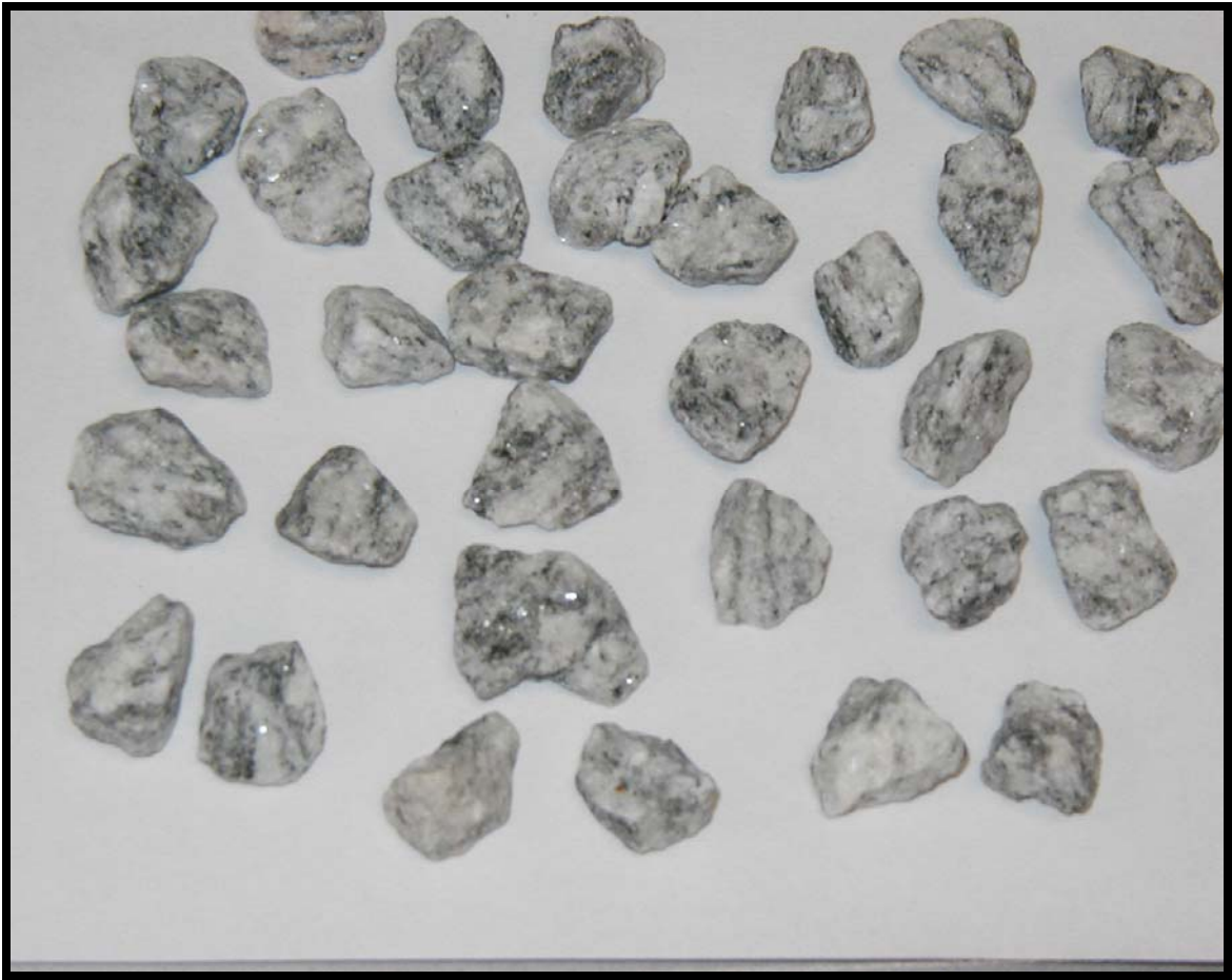
Figure D1. Georgia Granite Aggregate Particles-Granite-3 Passing 25 mm and Retained on 12.5 mm Sieve.
