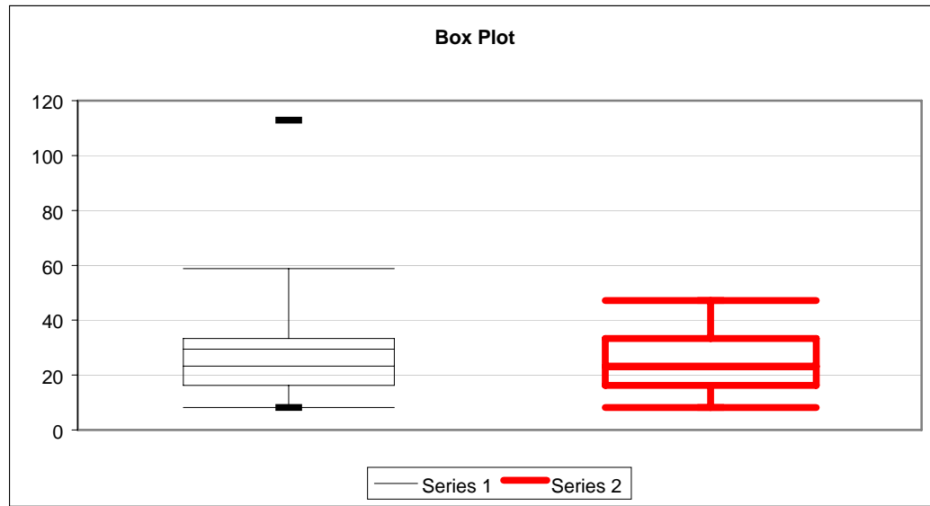
Figure 27. Box Plot: Angularity Values with and without Outliers.
