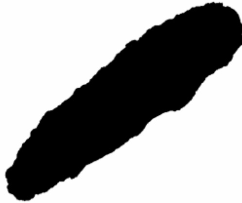
Figure 29. Elongated Aggregate with Very High Angularity and Form Value.
