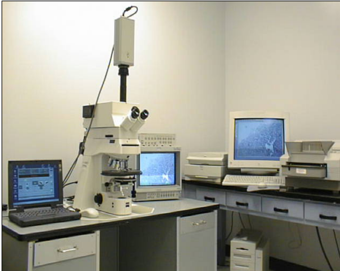
Figure 2. Image Acquisition System for Angularity and Form Index.
