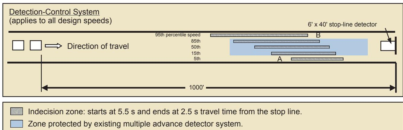
Figure 1. Detector Layout for the New Detection-Control System.
