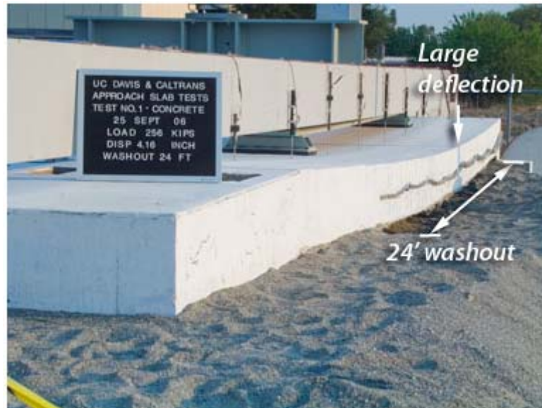
Figure 63 – Simulated Approach Slab Deflection Due to Washout by UC Davis Research Team
