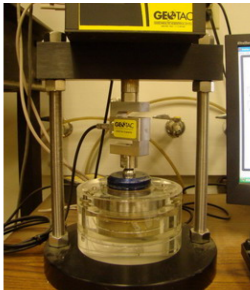
Figure 5.6. One-Dimensional Consolidation Test Setup.
