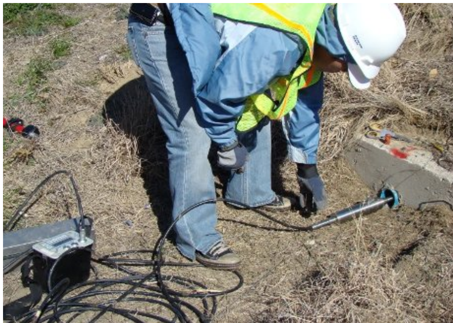
Figure 7.5. Inclinometer Data Collection Process.
