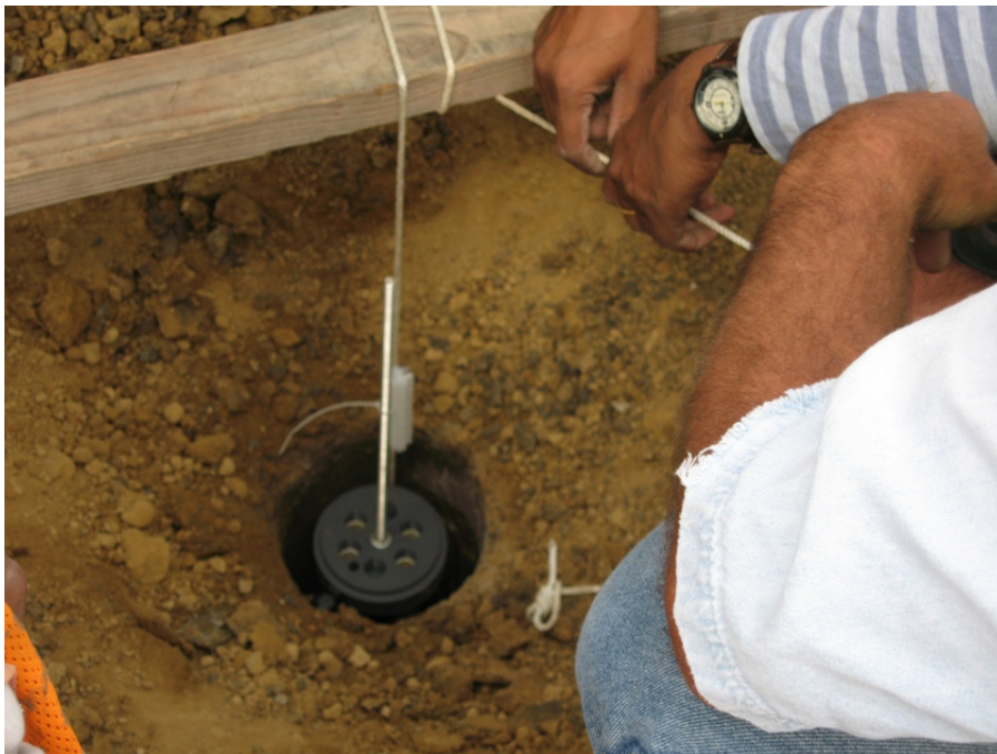
Figure 6.31. Set of Assembled Rods and Reference Head Held up by the Rope.
