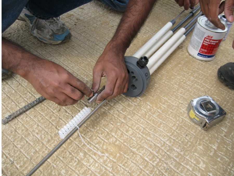
Figure 6.32. Placement of the VW Sensor Adapters into the Reference Head.
