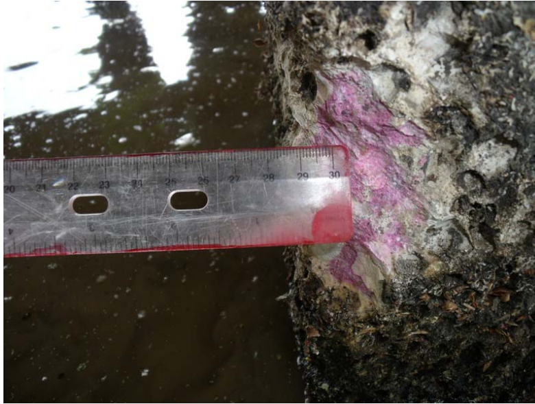
Figure 9. In Situ Phenolphthalein pH Test.
