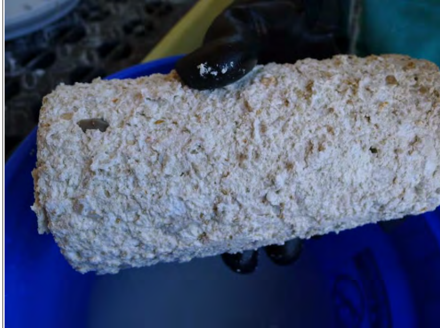
Figure F. 4. Reaction Products on the Surface of Specimen (C-I) after 83 days' Exposure in 3% Sulfuric Solution.
