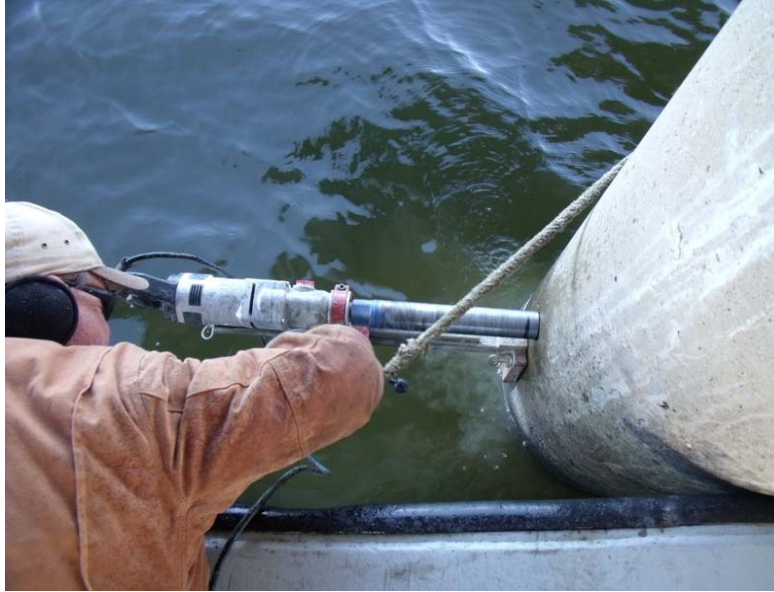
Figure 11. Core Specimen Collection.
