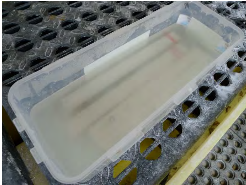
Figure F. 3. Storage of Mortar Specimen in Laboratory Simulation.
