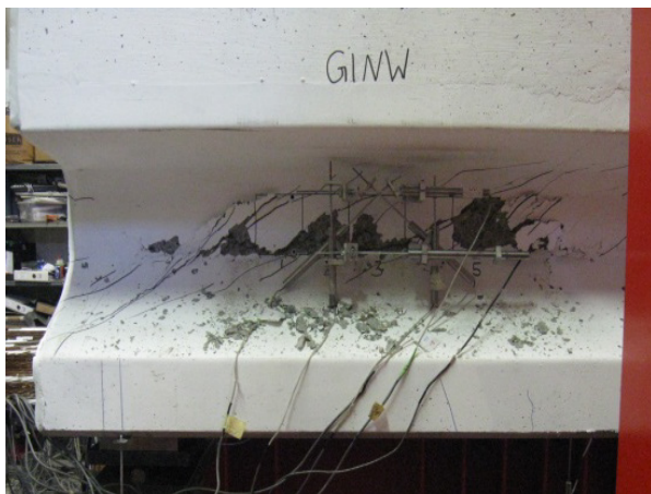
(e) Shear failure at 679.65 kips
