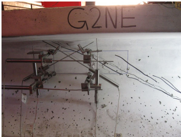
(c) Shear crack pattern before failure
