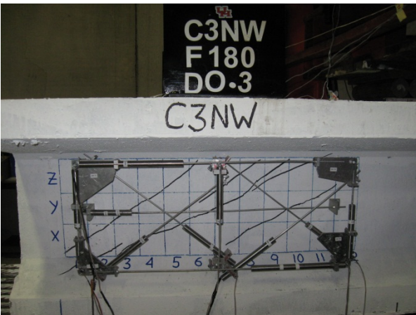
(c) Shear crack pattern before failure
