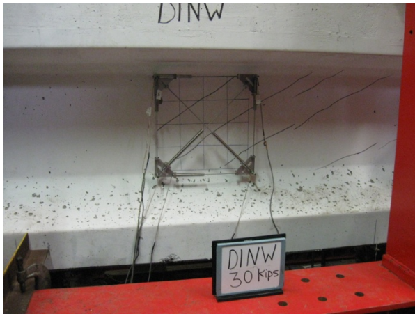
(a) Crack pattern at the start of north end testing
