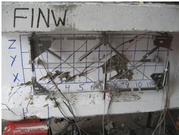
(e) Shear failure at 202.90 kips
