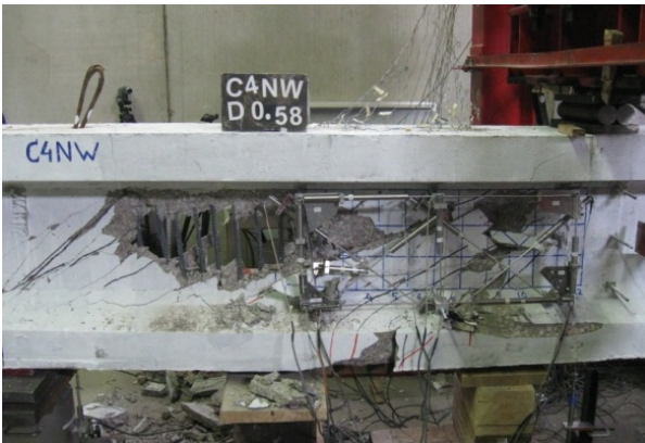
(e) Shear failure at 194 kips
