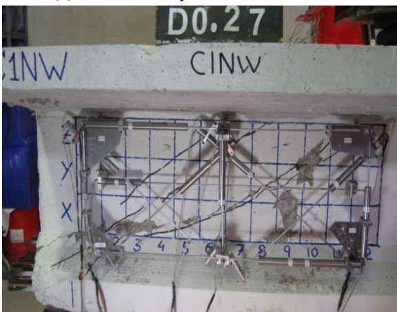
(e) Shear failure at 187.50 kips
