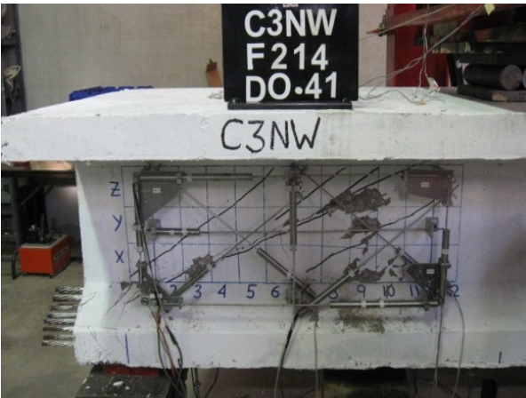
(e) Shear failure at 214.44 kips
