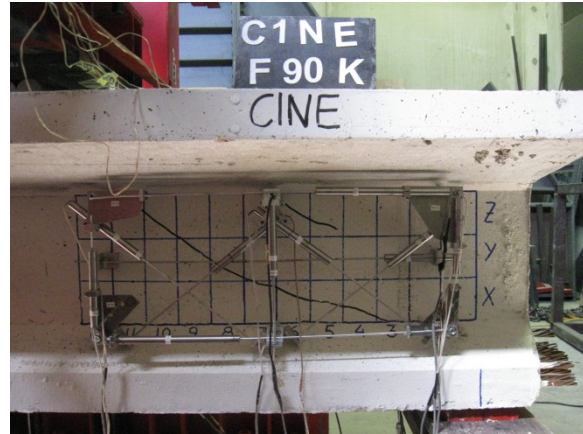
(b) First shear crack at 75 kips
