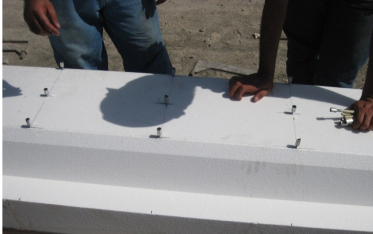
Fig. 3.16 Styro-Foam Forms with LVDT Rods
