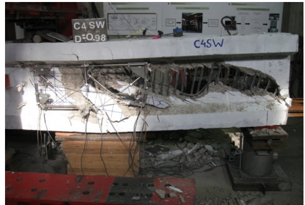
(f) Shear failure at 171.50 kips
