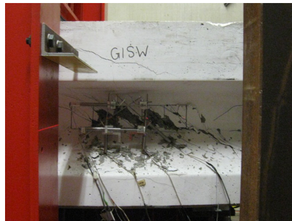
(f) Shear failure at 789.66 kips
