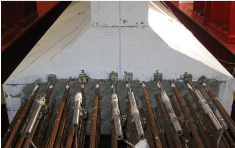
Fig. 6.23 LVDTs to Measure Slip
