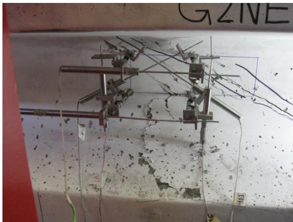
(e) Shear failure at 457.22 kips
