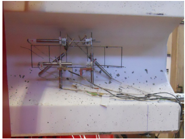
(b) First shear crack at 213 kips
