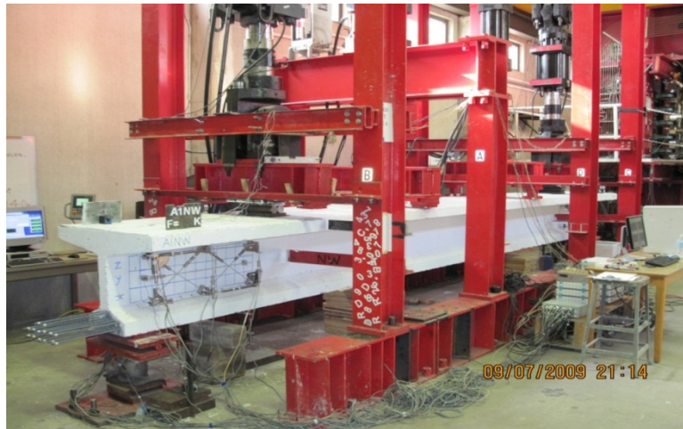
Fig. 3.21 Test Setup for Girders
