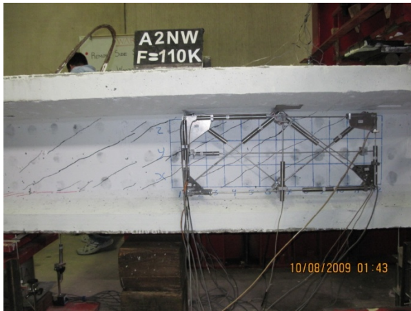
(c) Shear crack pattern before failure
