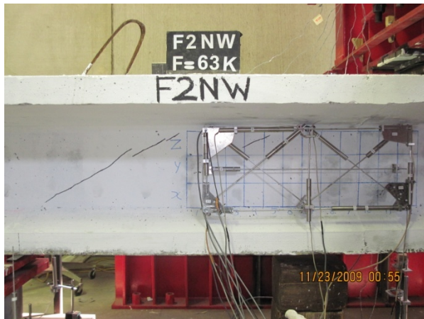
(a) First shear crack at 63 kips
