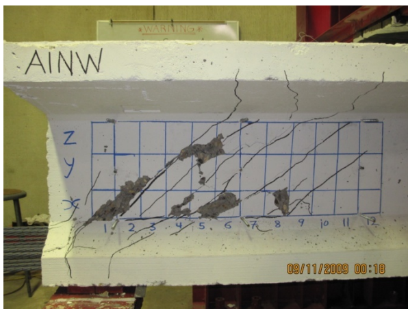
(e) Shear failure at 138.21 kips
