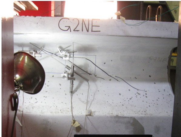
(a) First shear crack at 206 kips
