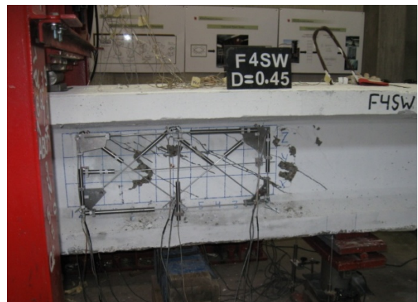
(f) Shear failure at 172.83 kips
