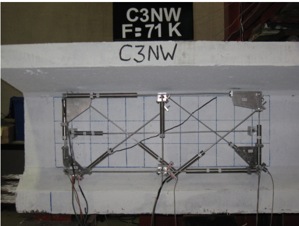
(a) First shear crack at 71 kips
