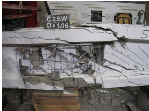
(f) Shear failure at 164.60 kips
