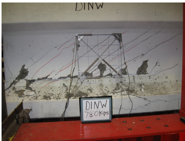
(e) Shear failure at 779.80 kips
