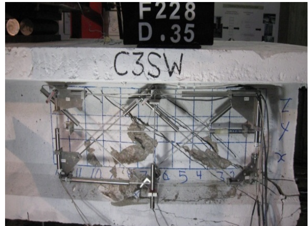
(f) Shear failure at 228.24 kips
