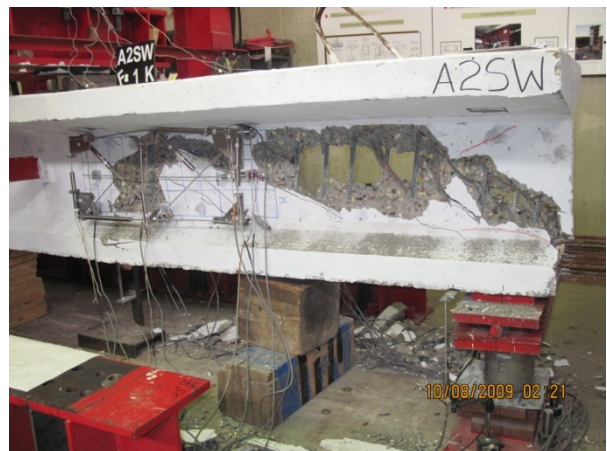
(f) Shear failure at 120.40 kips
