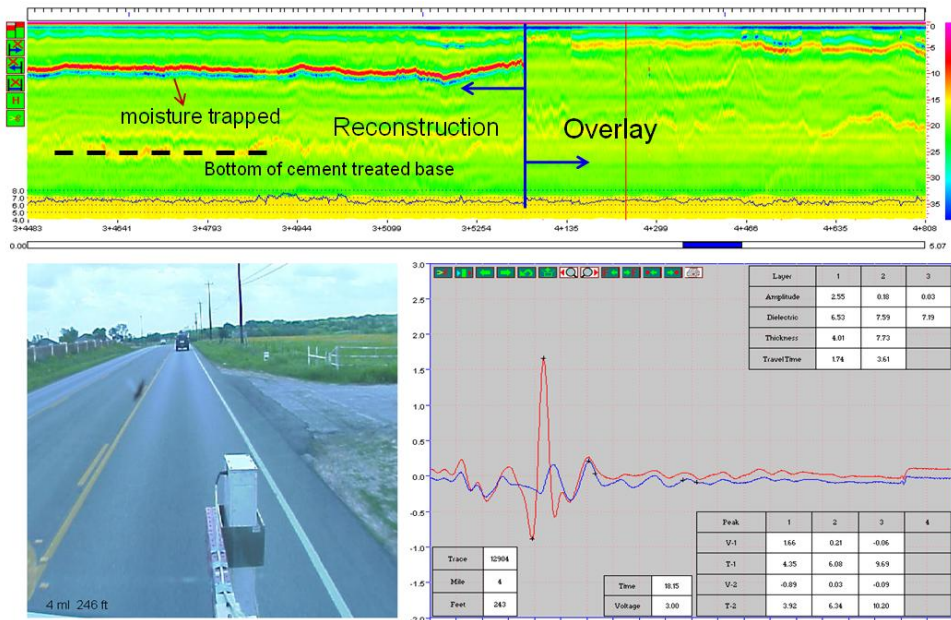
Figure 4.12. GPR Data between Reconstruction and Overlay Section.
