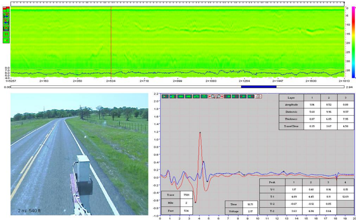
Figure C-3. GPR Data on Section 3 (Geogrid) of FM 1915.
