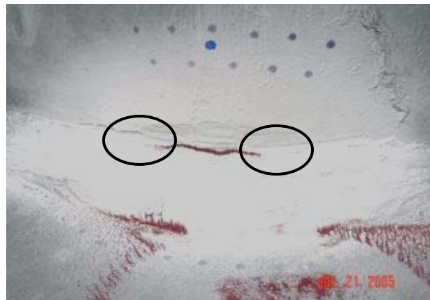
(d) Through-wall fracture revealed coterminous to lack of fusion (1/32" removal depth at weld toe)
