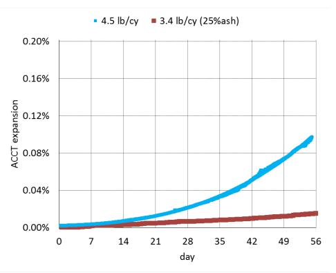
Figure 5.4. Expansion over Time for Mix 5 (s/c = 3).
