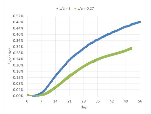
Figure 4.17. ACCT Using Mix 1 in Soak Solution Equal to Pore Solution with s/c = 3 and 0.27.
