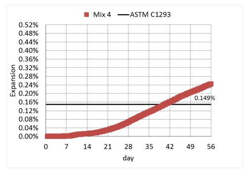
Figure 4.5. Expansion Curve of ACCT (Mix 4) over Time at Alkali Level of 4.5 lb/cy.
