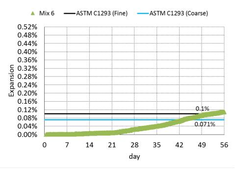
Figure 4.7. Expansion Curve of ACCT (Mix 6) over Time at Alkali Level of 4.5 lb/cy.
