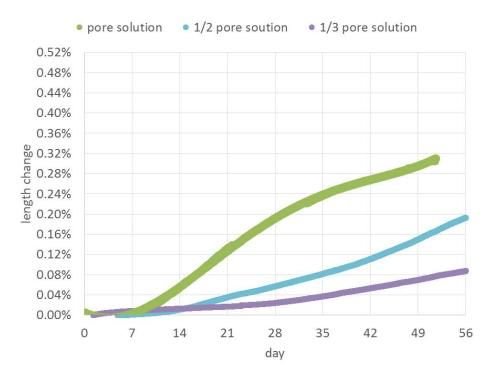
Figure 4.16. ACCT (s/c = 0.27) Using Mix 1 with Soak Solution Equal to Pore Solution, Soak Solution Equal to 1/2 of Pore Solution, and Soak Solution Equal to 1/3 of Pore Solution.
