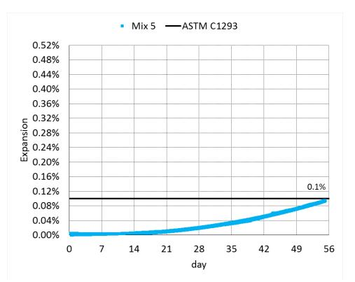
Figure 4.6. Expansion Curve of ACCT (Mix 5) over Time at Alkali Level of 4.5 lb/cy.
