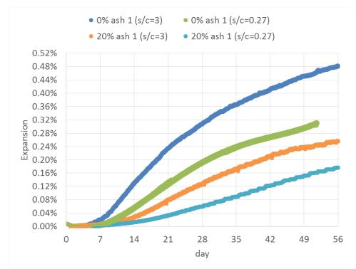
Figure 5.7. ACCT Using Mix 1 with and without Fly Ash Replacement (s/c = 3 and 0.27).
