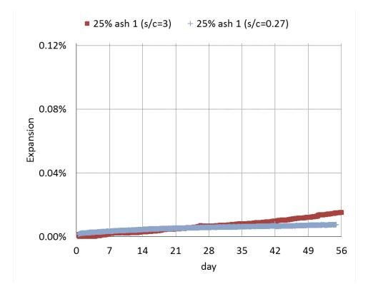
Figure 5.8. ACCT Using Mix 5 with Fly Ash Replacement (s/c = 3 and 0.27).
