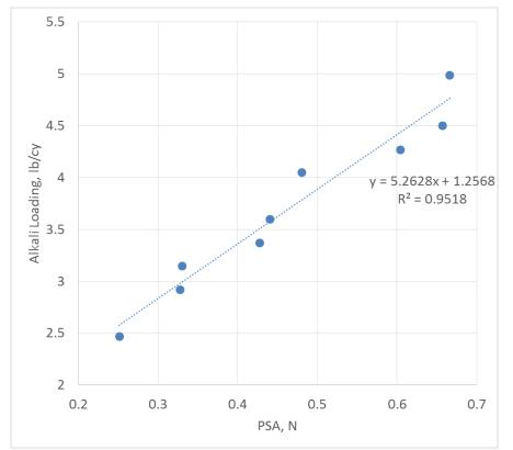
Figure 3.4. Correlation between Alkali Loading and PSA.
