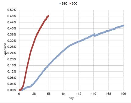
Figure 4.13. Effect of Temperature on ACCT (Mix 1) Expansion.
