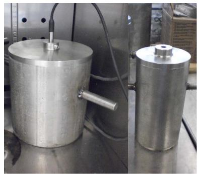
Figure 4.14. Two ACCT Setups Corresponding to Two Solution-to-Concrete Ratios: s/c = 3 (left) and s/c = 0.27 (right).
