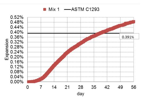
Figure 4.2. Expansion Curve of ACCT (Mix 1) over Time at Alkali Level of 4.5 lb/cy.
