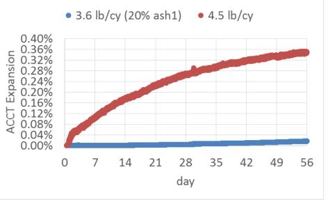
Figure 5.9. Expansion over Time for Mix 10 (s/c = 0.27).
