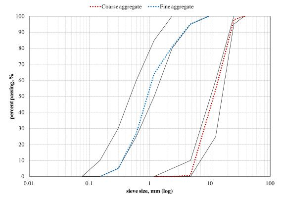
Figure 2.1. Gradation Curves of Aggregates.
