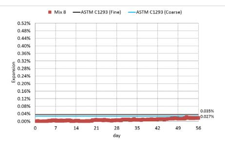
Figure 4.9. Expansion Curve of ACCT (Mix 8) over Time at Alkali Level of 4.5 lb/cy.
