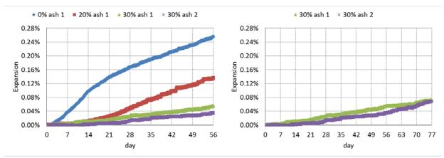
Figure 5.6. Expansion of Mix 7 with and without Fly Ash Replacement (left) and Tested with Fly Ash for a Long Period of Time (right) (s/c = 3).
