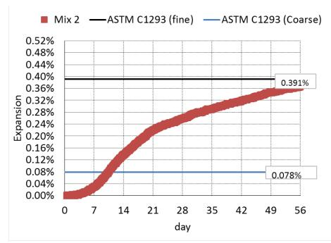
Figure 4.3. Expansion Curve of ACCT (Mix 2) over Time at Alkali Level of 4.5 lb/cy.
