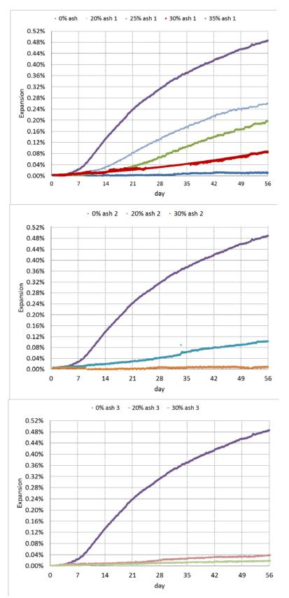
Figure 5.1. Expansion of Mix 1 with and without Fly Ash Replacement (s/c = 3).
