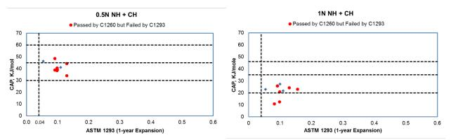
Figure 3.2. Correlation between CAP of Aggregate and ASTM C1293.
