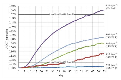
Figure 5.2. Expansion of Mix 1 with Fly Ash 1 Replacement for a Long Period of Time (s/c = 3).
