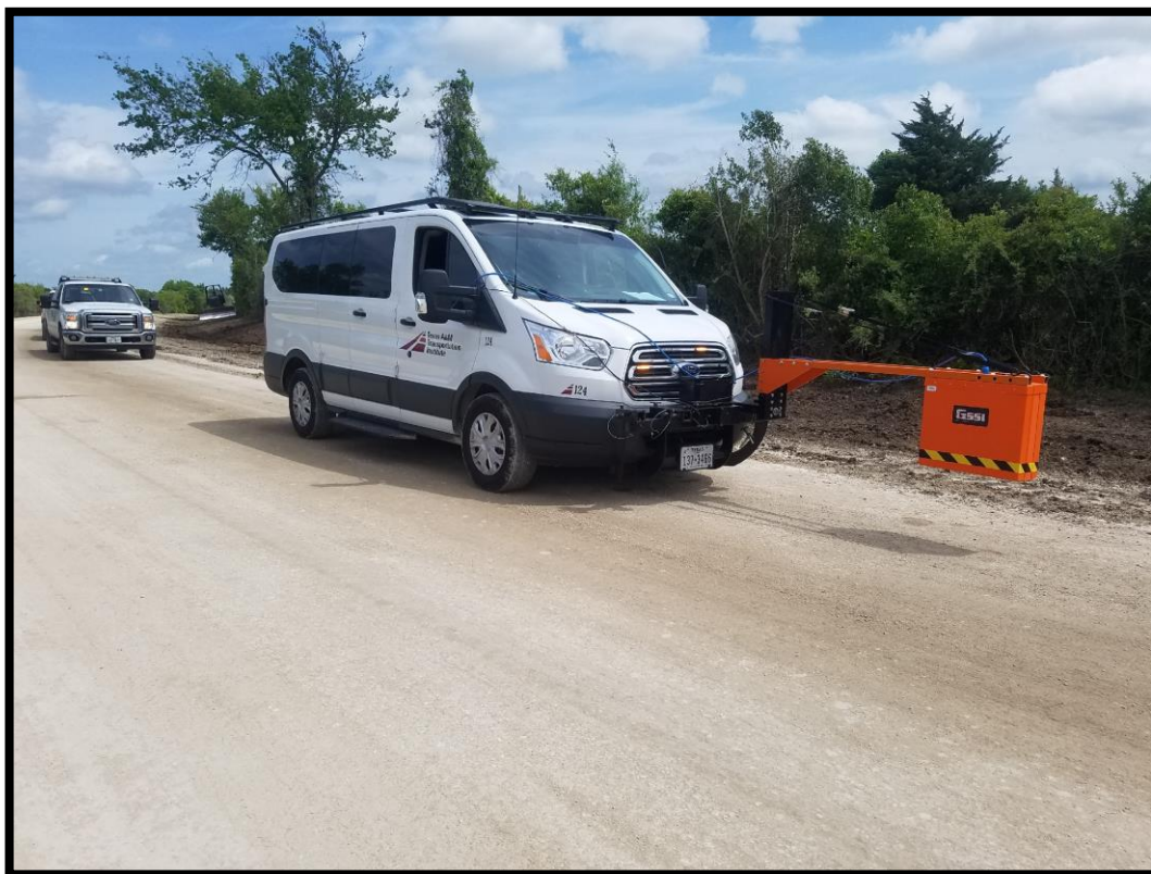
GPR testing on Completed Base Course
