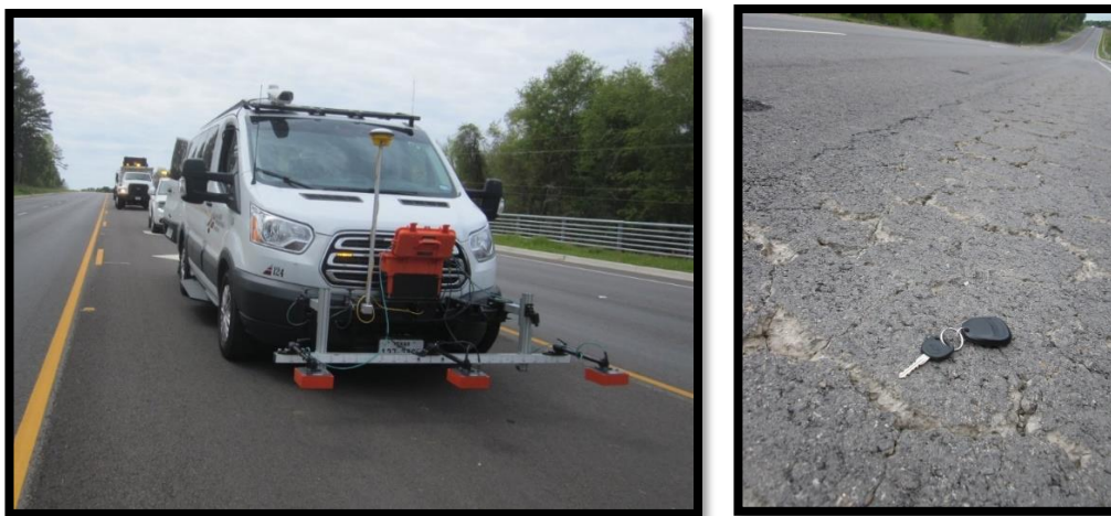
Figure 39. Using GPR for Forensic Investigation.
