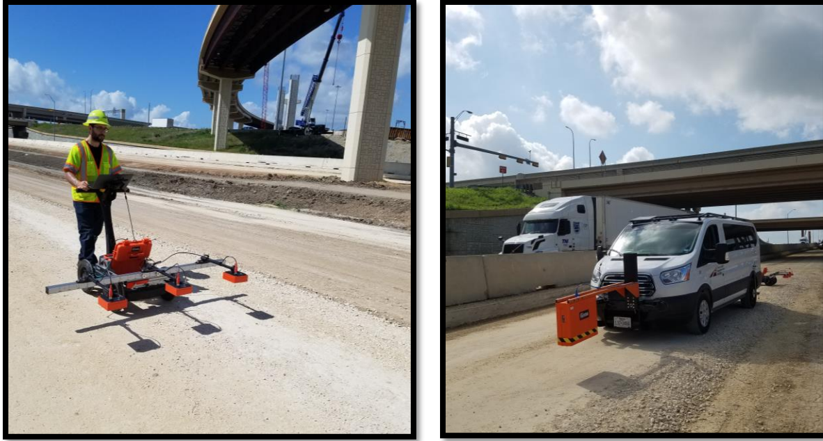
Figure 11. GPR Collection on SH 130 for Mechanics-Based Models.
