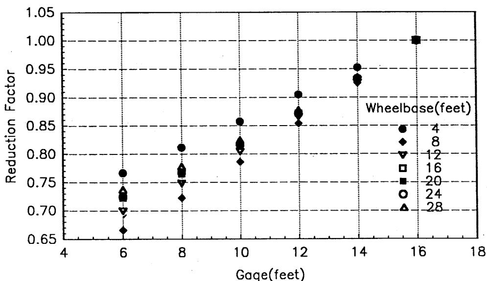
Figure 15: Reduction Factor versus Gage for Wheelbases Ranging from 4 to 28 ft.
