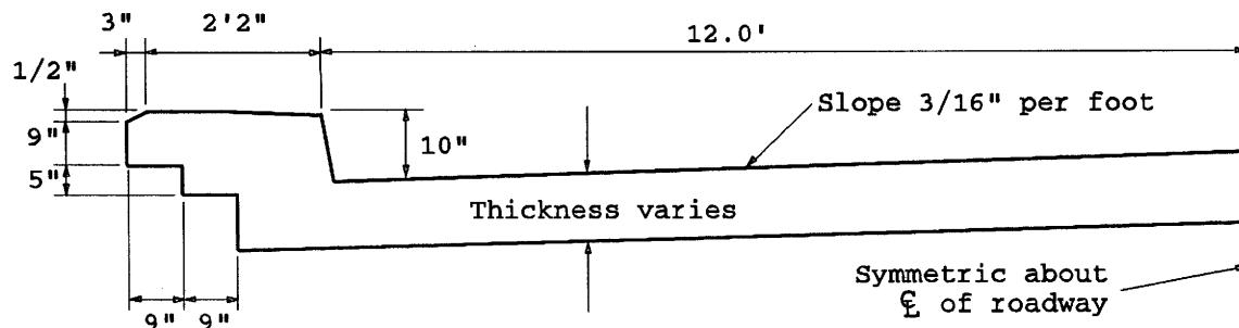
Figure 6: Typical H15 simple span reinforced concrete bridge.
