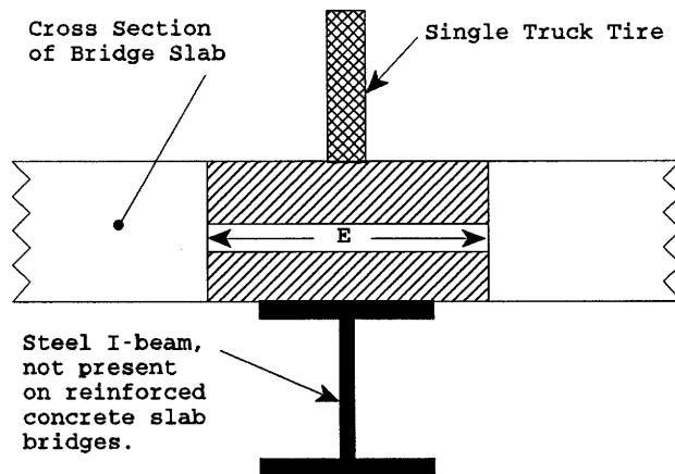
Figure 8: Illustration of Distribution Factor E.
