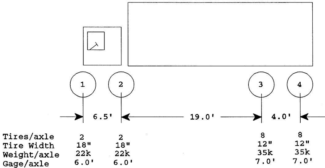
**Figure 2:** Overweight vehicle configuration example.
