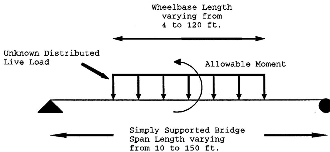
Figure 5: Unknown distributed load illustration.
