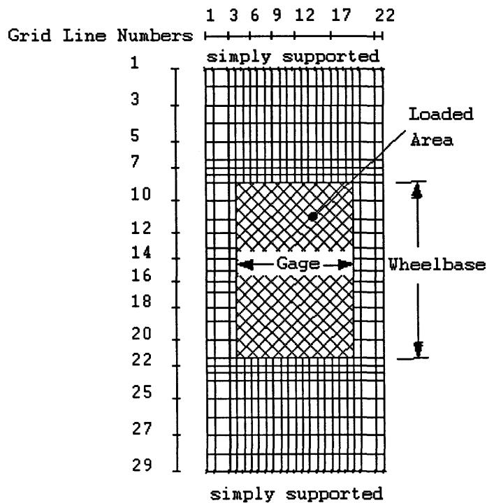
Figure 14: Typical finite element mesh for a concrete slab bridge used with SAFE.
