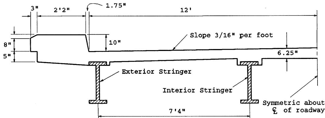
Figure 7: Typical H15 simple span steel I-beam bridge.
