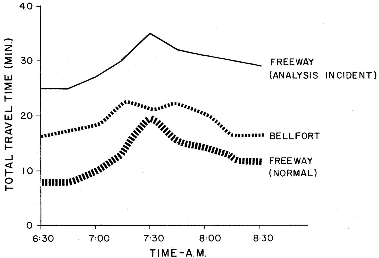
FIGURE 19 - TRAVEL TIME ON BELLFORT ALTERNATE ROUTE AND ON FREEWAY - 6:30-8:30A.M.
