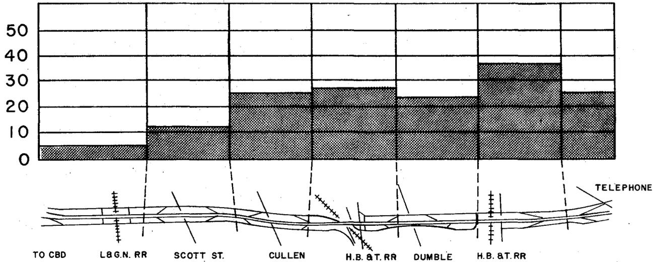
FIGURE 5 - DISTRIBUTION OF ACCIDENTS AND STALLED VEHICLES ON INBOUND GULF FREEWAY 6:30 - 9:00 AM AND 4:30 - 6:00 PM
