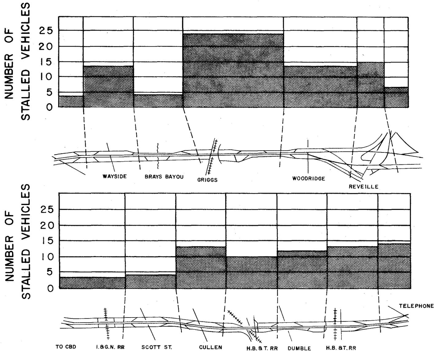
FIGURE 4 - DISTRIBUTION OF STALLED VEHICLES ON INBOUND GULF FREEWAY - 6:30-9:00 AM AND 4:30-6:00 PM
