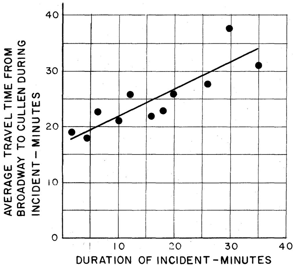
**FIGURE 9 - AVERAGE TRAVEL TIME FROM BROADWAY TO CULLEN DURING INCIDENTS OF VARYING DURATION FROM 6:30 - 8:30 A.M.**
