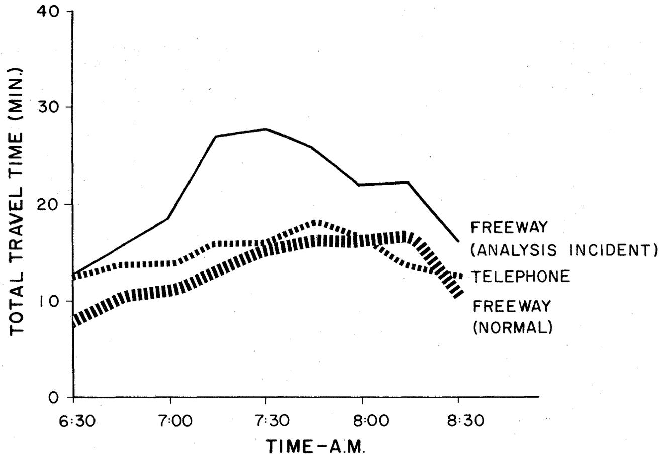
FIGURE 23— TRAVEL TIME ON TELEPHONE ALTERNATE ROUTE AND ON FREEWAY — 6:30-8:30A.M.
