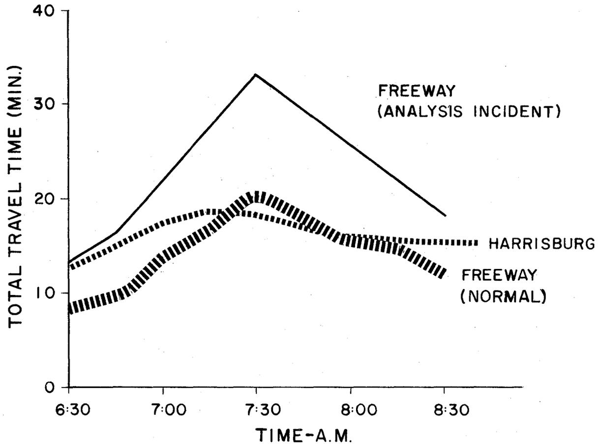
FIGURE 13 - TRAVEL TIME ON HARRISBURG ALTERNATE ROUTE AND ON FREEWAY - 6:30-8:30A.M.
