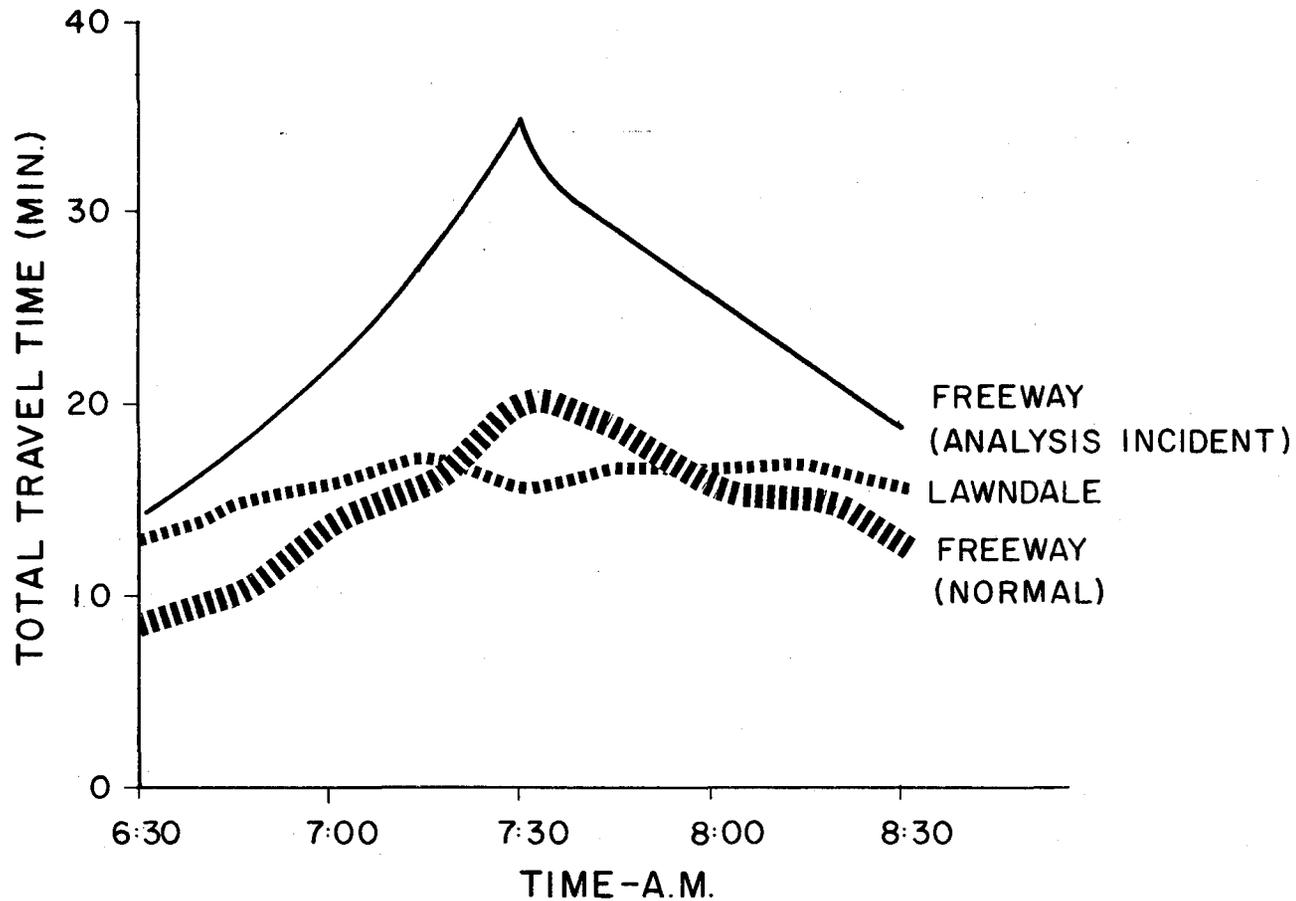
FIGURE 17 - TRAVEL TIME ON LAWNDALE ALTERNATE ROUTE AND ON FREEWAY - 6:30 - 8:30 A.M.
