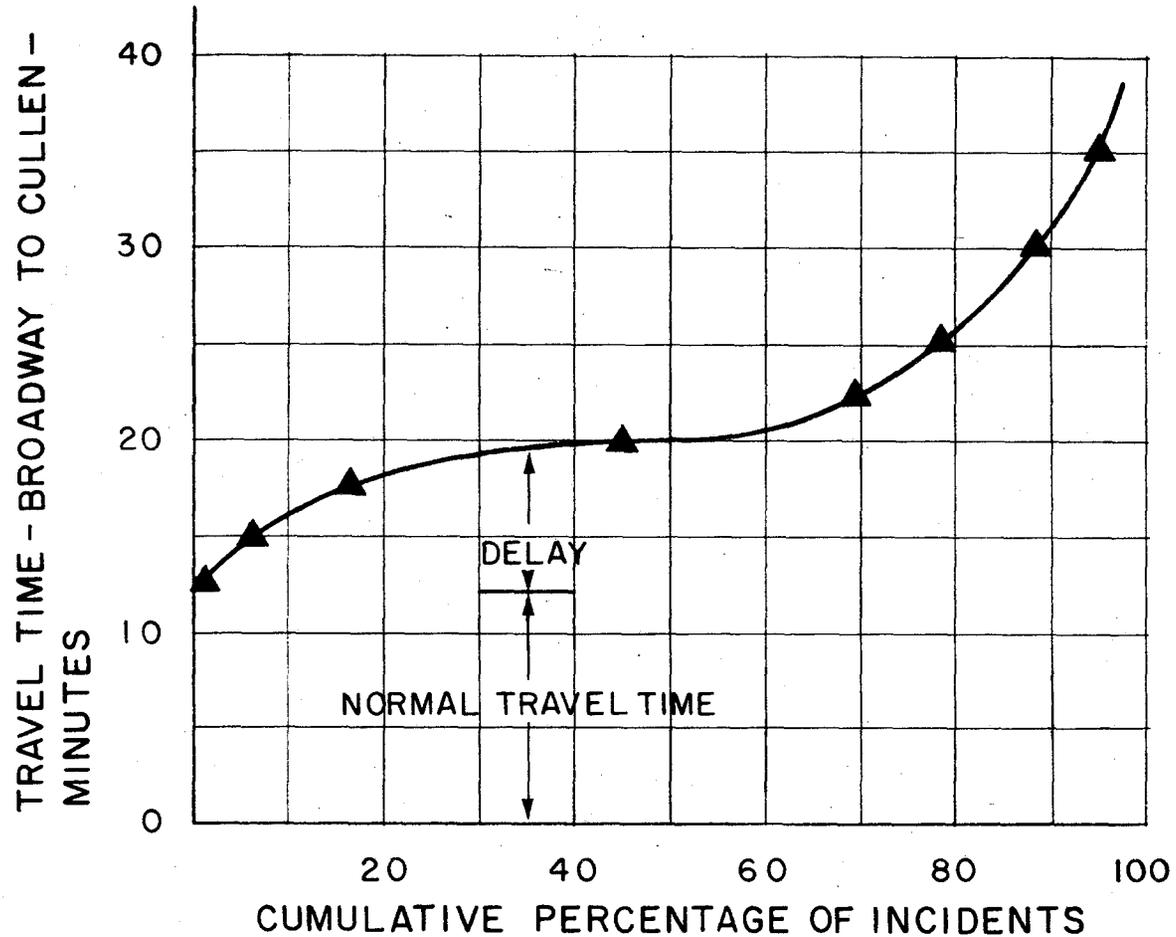
**FIGURE 10 - TRAVEL TIME AND DELAY FROM BROADWAY TO CULLEN AS RELATED TO INCREASING SEVERITY OF INCIDENTS FROM 6:30 - 8:30 A.M.**
