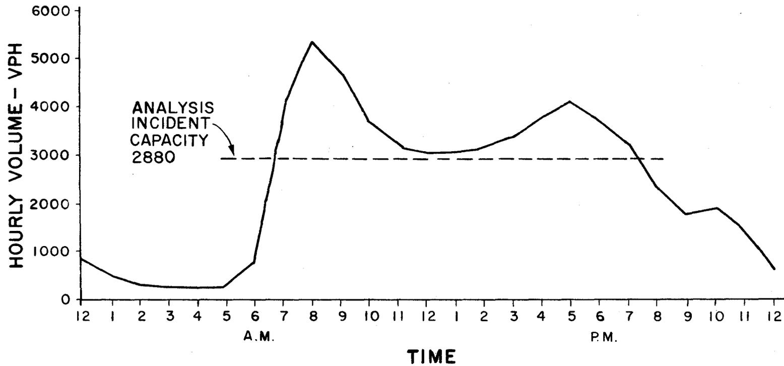
FIGURE 6 - INBOUND GULF FREEWAY INCIDENT CAPACITY AND 24-HOUR VOLUMES AT GRIGGS OVERPASS
