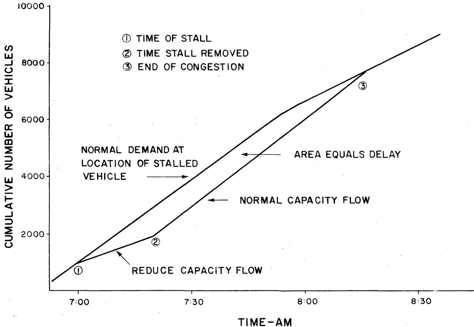
**FIGURE 8— EXAMPLE OF DELAY CAUSED BY A STALLED VEHICLE BLOCKING ONE LANE AT 7A.M. ON INBOUND GULF FREEWAY**
