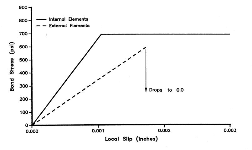
Figure 2.5. Recommended Linear Approximations for the Bond Stress-Slip Relationship for Tensile Specimens from Wahla (<u>10</u>).
