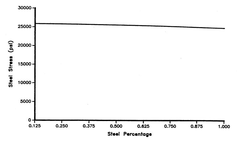
Figure 5.12. Steel Stress at Crack vs. Steel Percentage.
