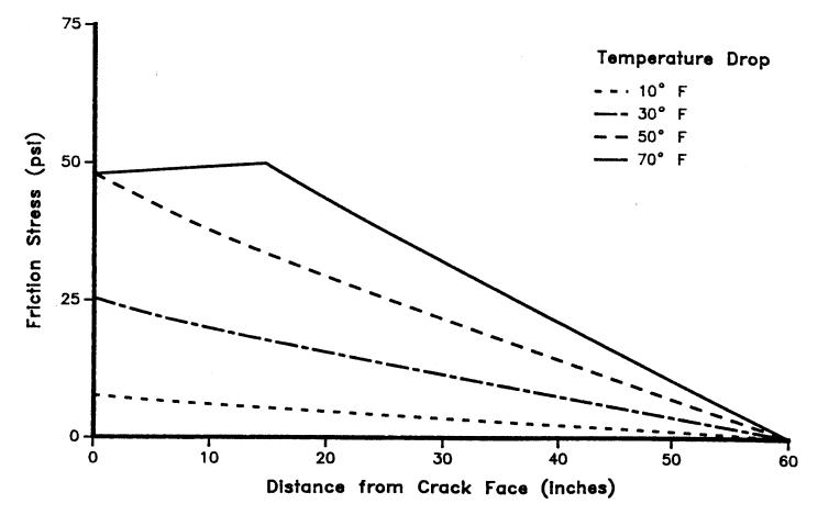
Figure 5.20. Friction Stress Distributions at Temperature Drops of 10°, 30°, 50°, and 70°F.
