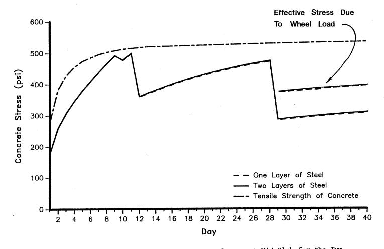
Figure 5.25. Variation of the Concrete Stress at Mid-Slab for the Two Pavements over the Analysis Period, with the Effective Stress Due to Wheel Loading Shown.
