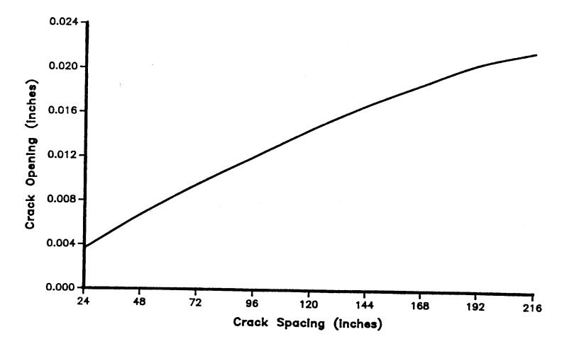
Figure 5.16. Crack Opening vs. Crack Spacing.
