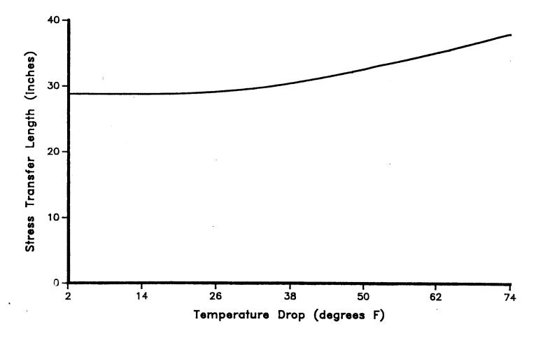
Figure 5.18. Stress Transfer Length vs. Temperature Drop.
