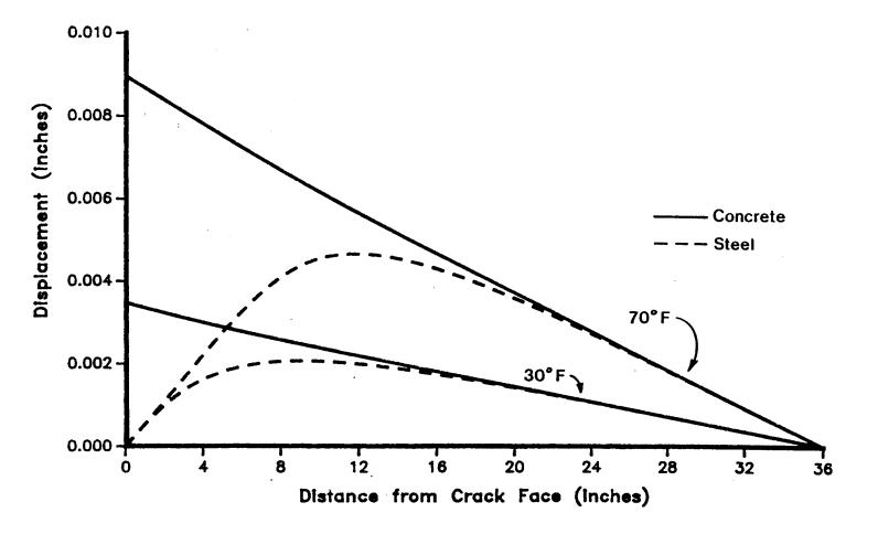
Figure 5.5. Concrete and Steel Displacement Distributions at Temperature Drops of 30° and 70°F.
