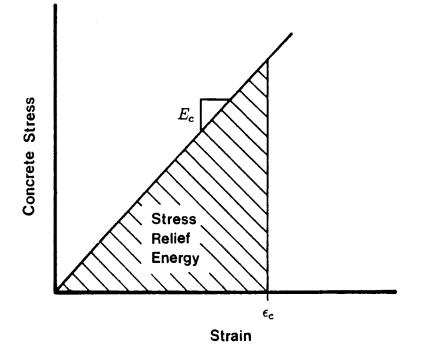
Figure 4.3. Stress Relief Energy Lost by the Concrete at a Strain  $\epsilon_c$ .
