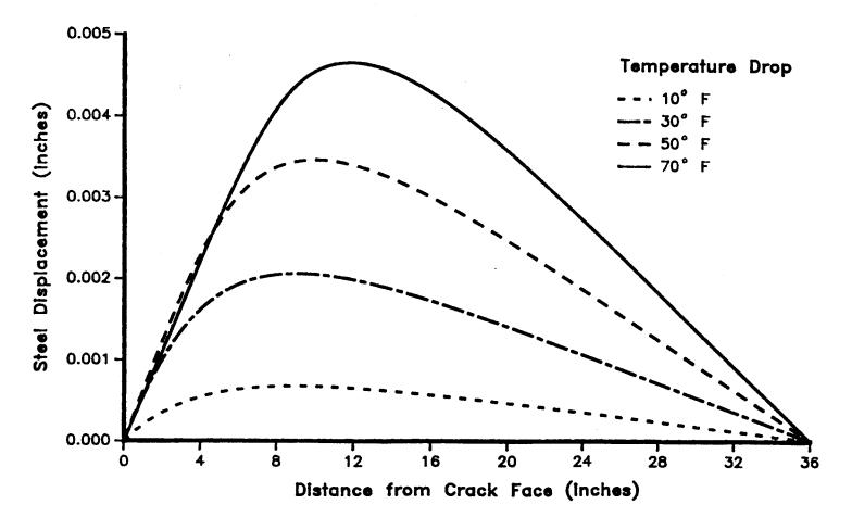
Figure 5.4. Steel Displacement Distributions at Temperature Drops of 10°, 30°, 50°, and 70°F.
