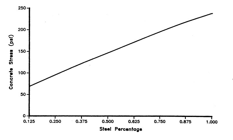
Figure 5.11. Concrete Stress at Mid-Slab vs. Steel Percentage.
