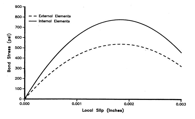
Figure 2.4. Experimental Bond Stress vs. Slip Curves for Tensile Specimens from Wahla (<u>10</u>).
