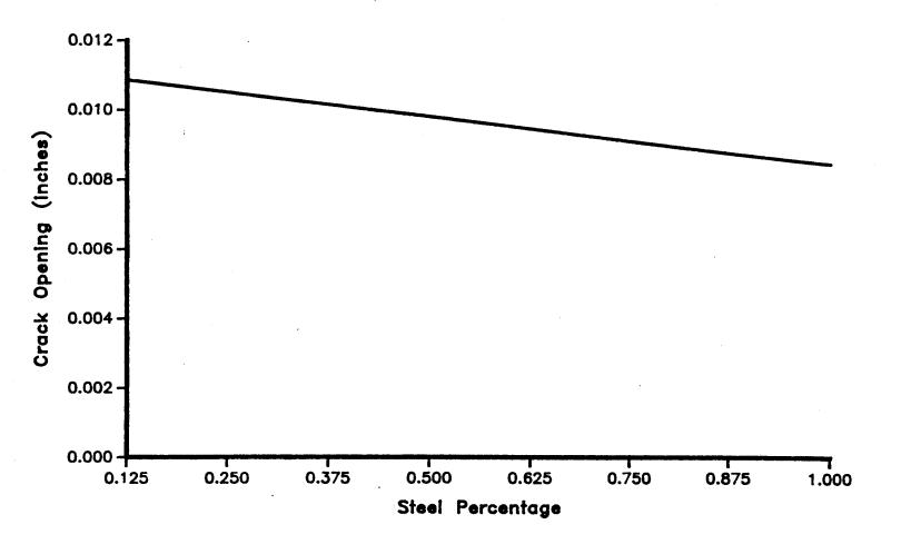
Figure 5.13. Crack Opening vs. Steel Percentage.
