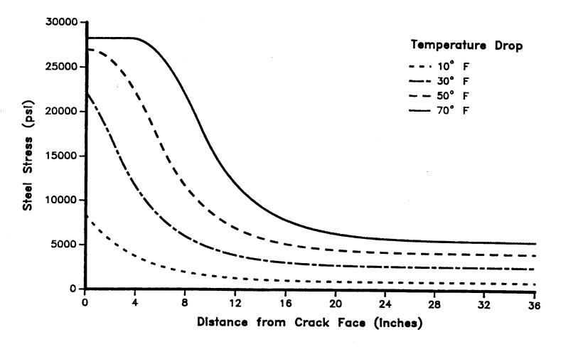
Figure 5.7. Steel Stress Distributions at Temperature Drops of 10°, 30°, 50°, and 70°F.
