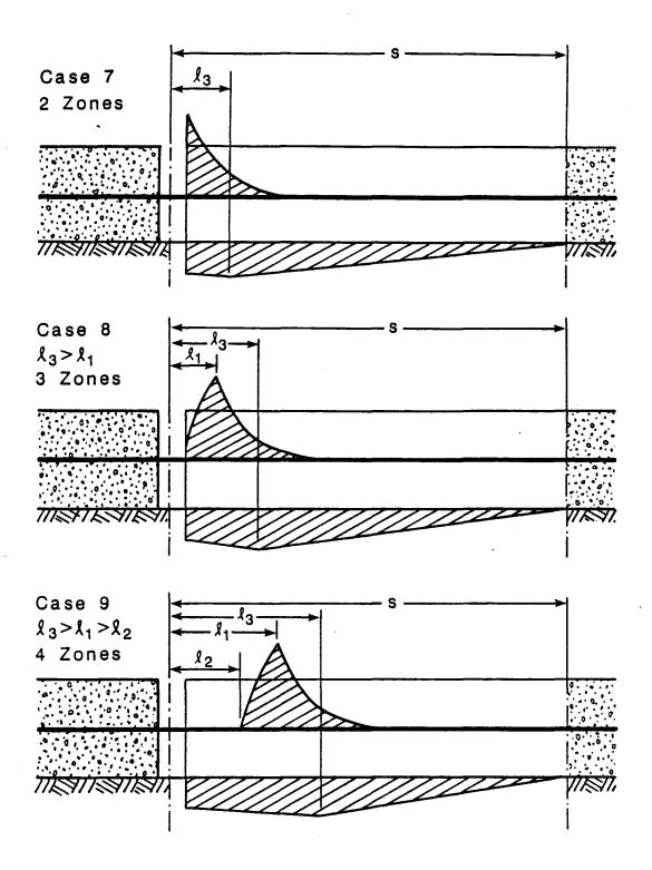
Figure 3.5c. Cases Describing the Different Combinations of the Bond Stress and Friction Stress Distributions. Cases 7 through 9.
