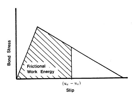
Figure 4.2a. Frictional Work Energy Expended Between the Steel and the Concrete to Achieve a Relative Slip of  $(u_c - u_s)$ .
