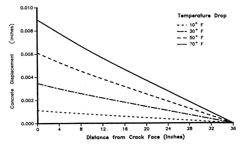
Figure 5.3. Concrete Displacement Distributions at Temperature Drops of 10°, 30°, 50°, and 70°F.
