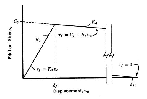
Figure 3.4b. The Friction Stress Function.
