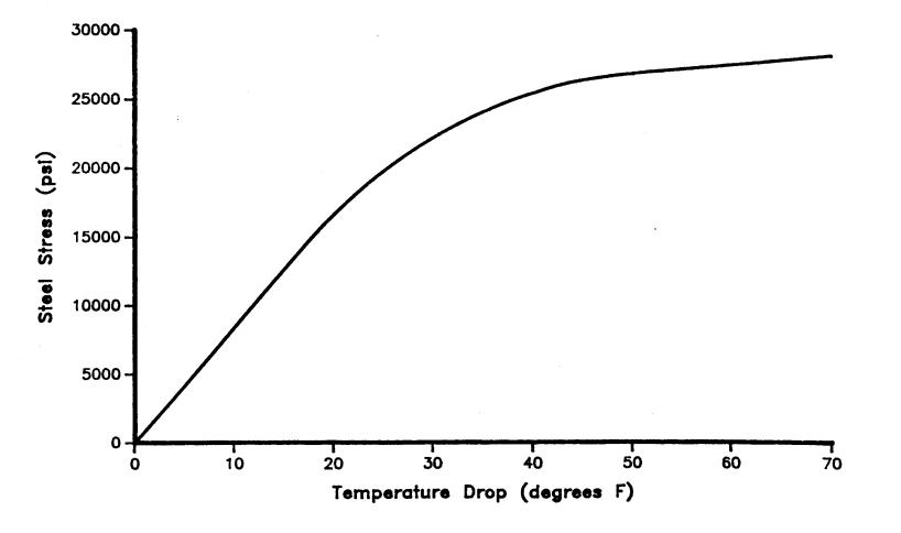
Figure 5.9. Steel Stress at Crack vs. Temperature Drop.
