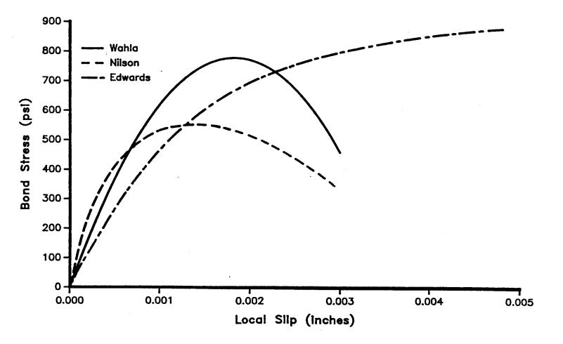
Figure 2.6. Comparison of Experimental Bond Stress vs. Slip Curves (<u>10</u>, <u>11</u>, <u>12</u>).
