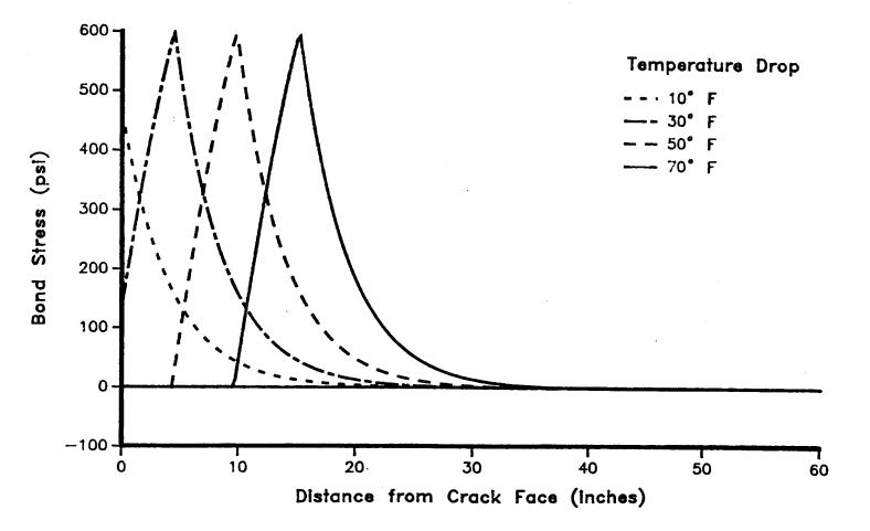
Figure 5.19. Bond Stress Distributions at Temperature Drops of 10°, 30°, 50°, and 70°F.
