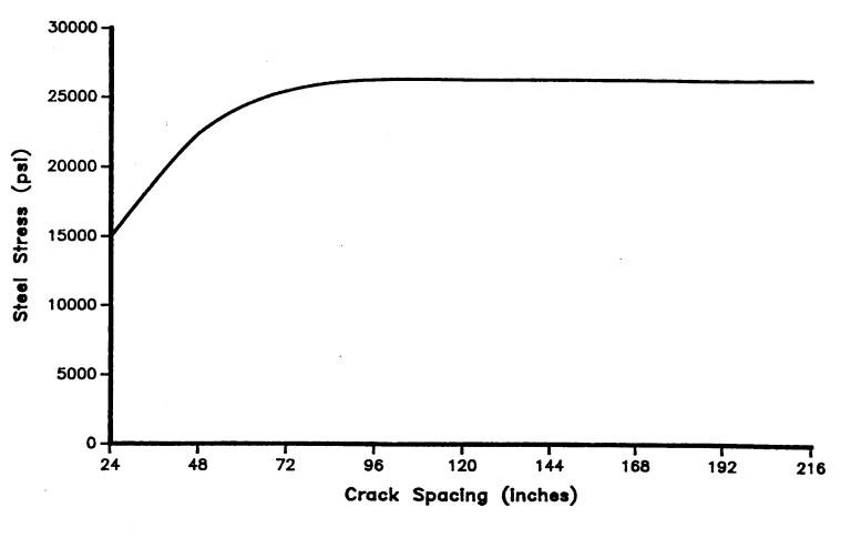
Figure 5.15. Steel Stress at Crack vs. Crack Spacing.
