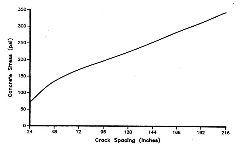
Figure 5.14. Concrete Stress at Mid-Slab vs. Crack Spacing.
