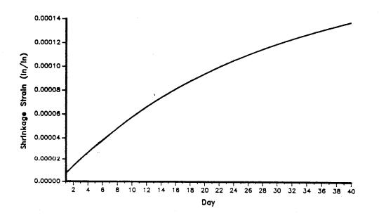
Figure 5.21b. Shrinkage Strain Distribution for the 40 Day Analysis Period.
