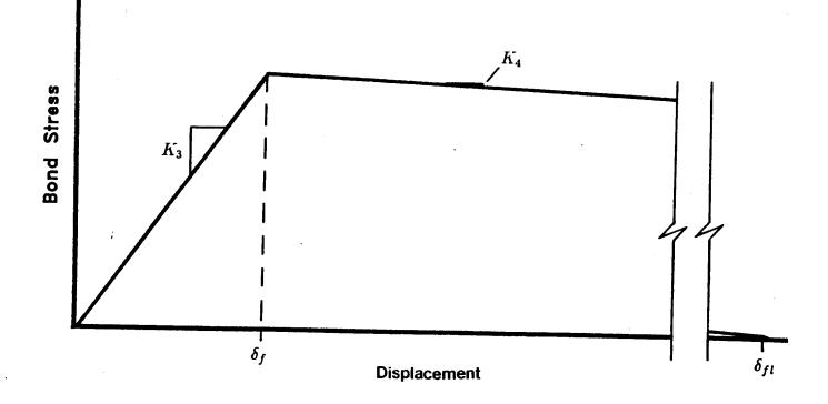
Figure 2.10. Proposed Friction Stress Function.
