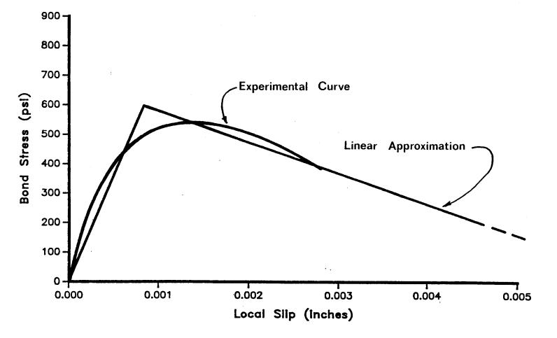
Figure 2.8. Bond Stress Function and Experimental Bond Stress vs. Slip Curve from Nilson (<u>11</u>).
