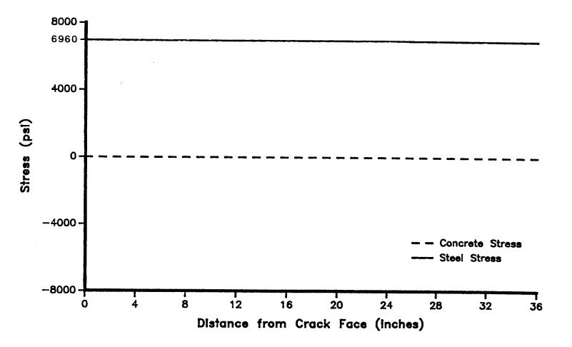
Figure 5.2. Concrete and Steel Stress Distributions for Zero Friction Test Case.
