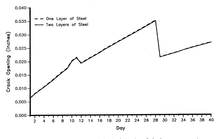
Figure 5.23. Variation of the Crack Opening of the Pavements over the Analysis Period.
