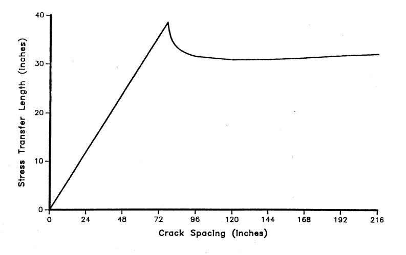
Figure 5.17. Stress Transfer Length vs. Crack Spacking.
