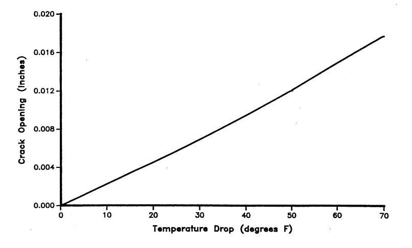
Figure 5.10. Crack Opening vs. Temperature Drop.
