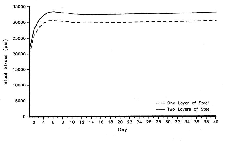
Figure 5.24. Variation of the Steel Stress at the Crack for the Two Pavements over the Analysis Period.
