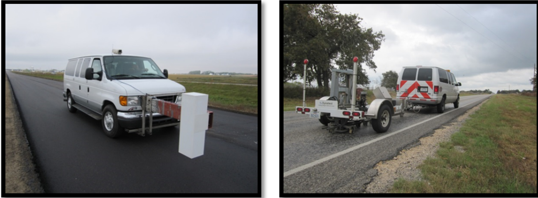
Figure 3. GPR and FWD Testing.
