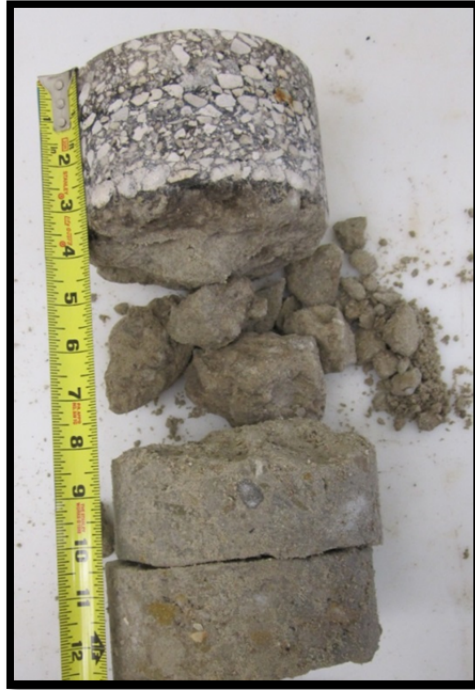
Figure 6. Coring to Help Determine Layer Condition.
