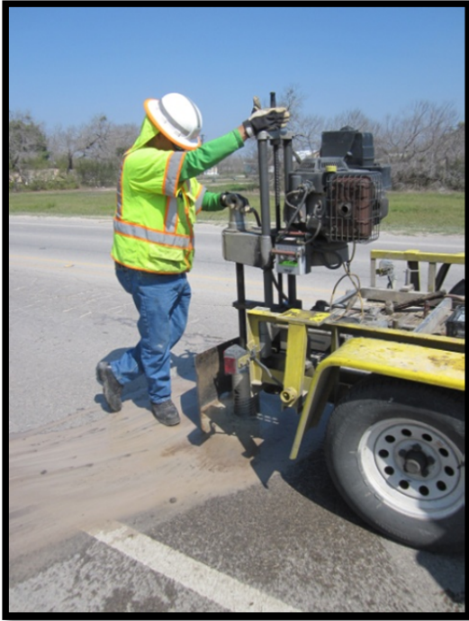
Figure 6. Coring to Help Determine Layer Condition.
