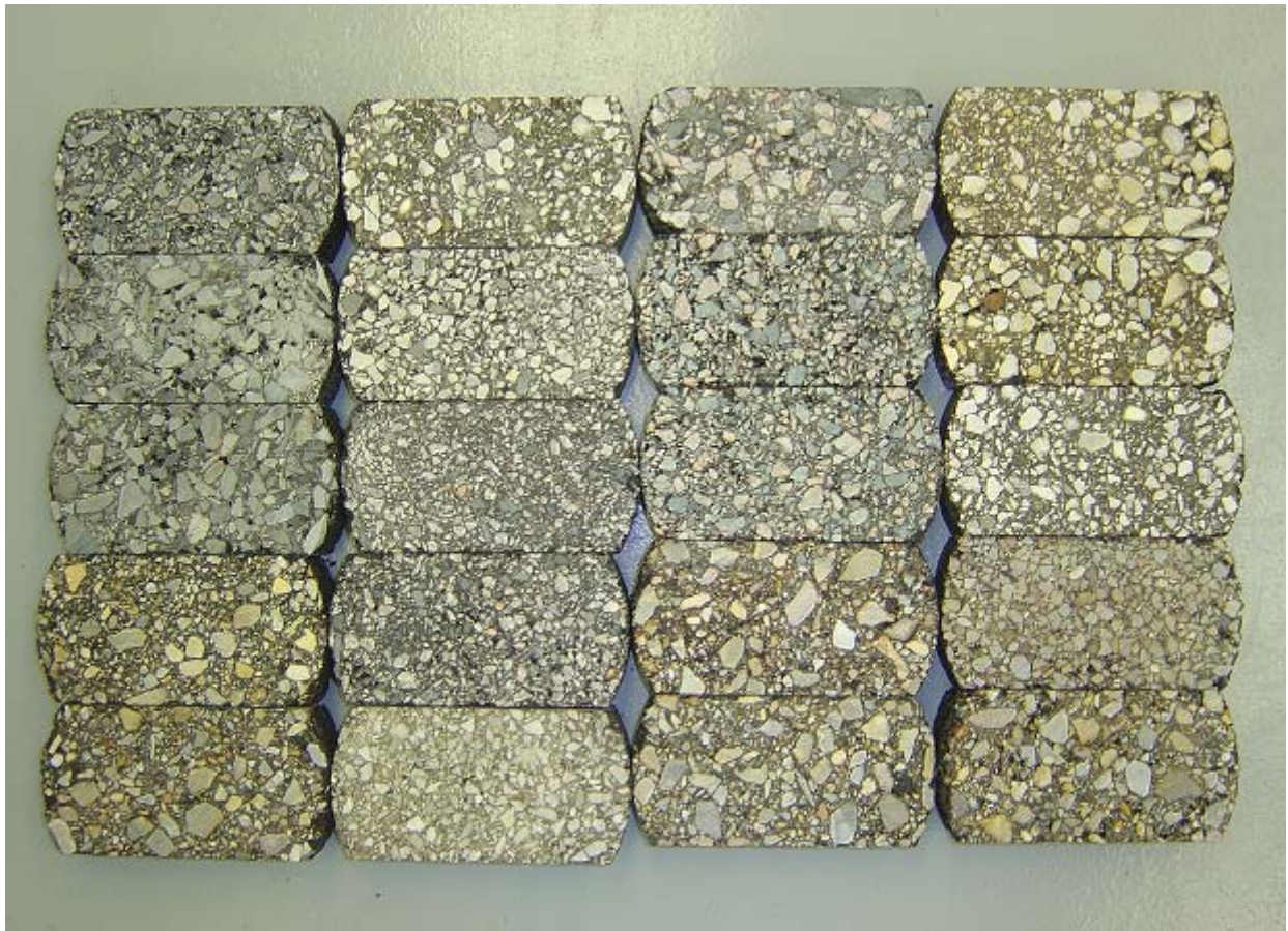
Figure 8. OT Specimens Cut from Double-Blade Saw.
