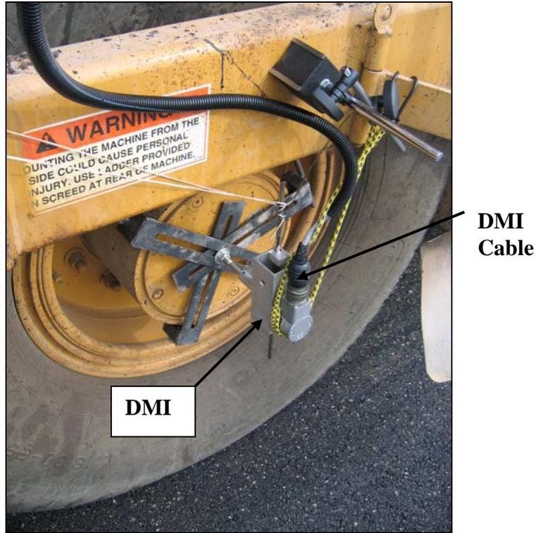
**Figure 8. Installed DMI.**
