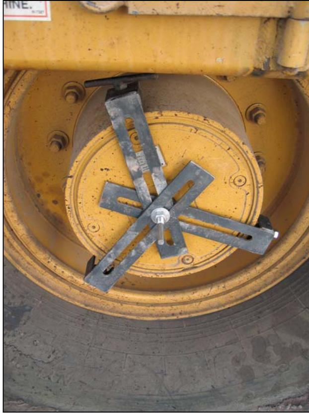
**Figure 4. DMI Mount Attached to Paver Wheel Hub.**
