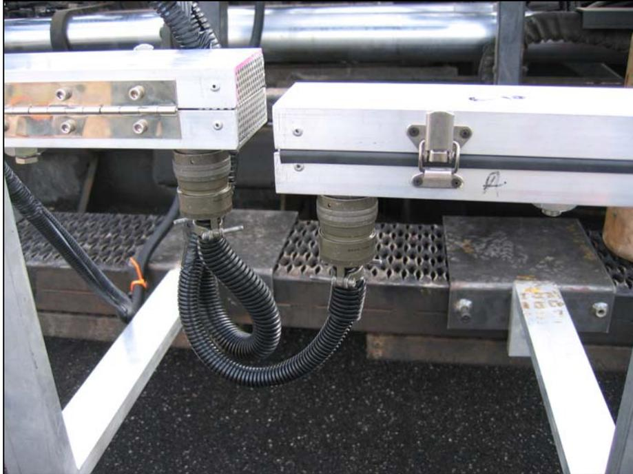
**Figure 6. Master Control Cable Connected to IR Bars.**
