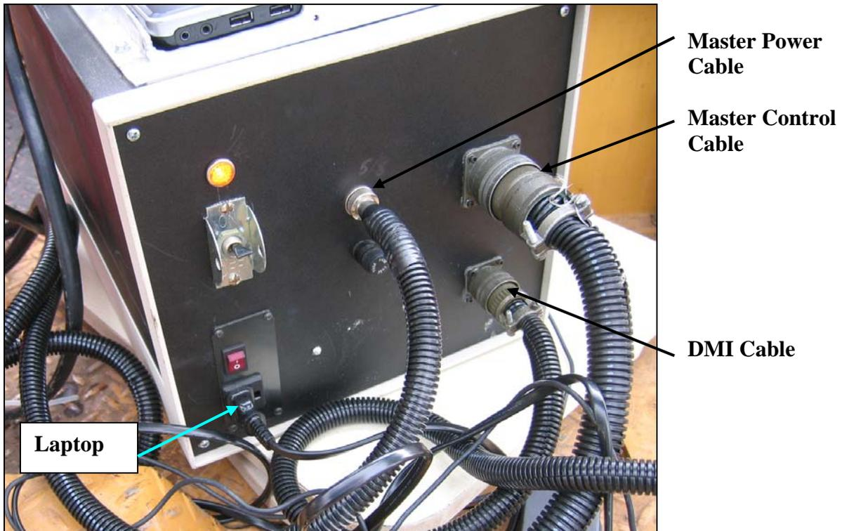
**Figure 7. Proper Connections at Master Control Box.**
