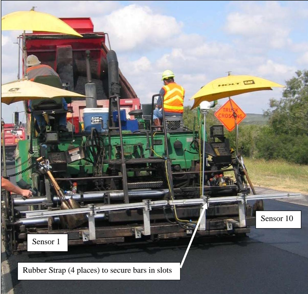
**Figure 5. IR Bar Mounts with IR Bars Installed.**
