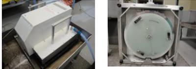
The dynamic friction test is used to measure friction in a spot location at variable speeds and can be used along with CTM to predict skid number (SN).
