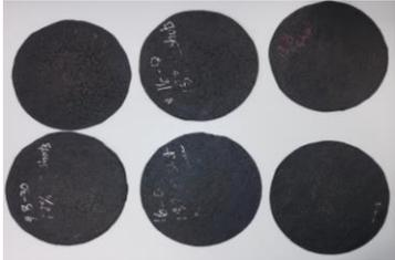
The procedure included pouring of the slurry into the circular opening of a template resting on roofing felt, followed by oven curing at 60C for 24 hrs. The specimen was soaked in water for one hour and after that mechanically abraded underwater with a rubber hose for 5 minutes and 15 seconds.
