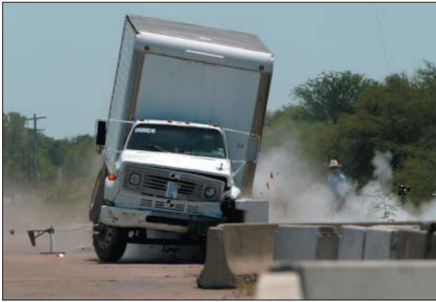
Figure 3. NCHRP Report 350 test 4-12 on the TxDOT F411 bridge rail.
