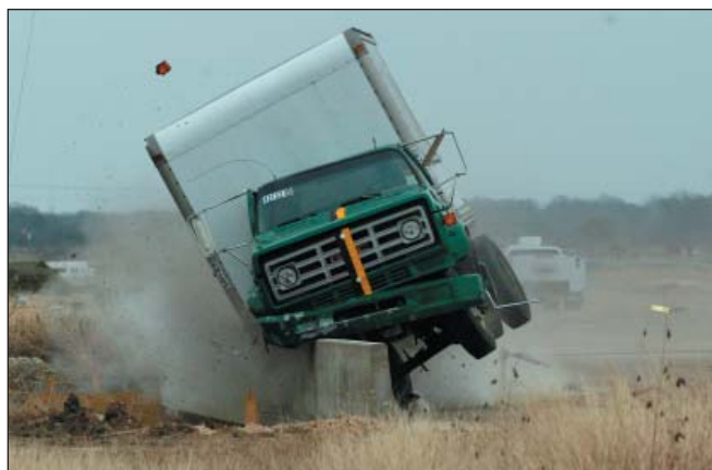
Figure 1. NCHRP Report 350 test 4-12 on the 32-inch (813 mm) Jersey-shaped railing design used in Florida.
