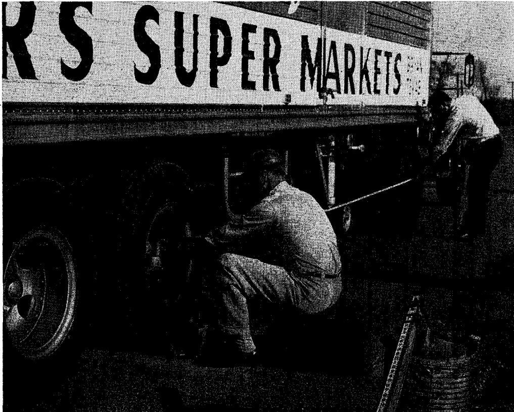
Figure 14 — Measuring wheel base between axles 2 and 3.
