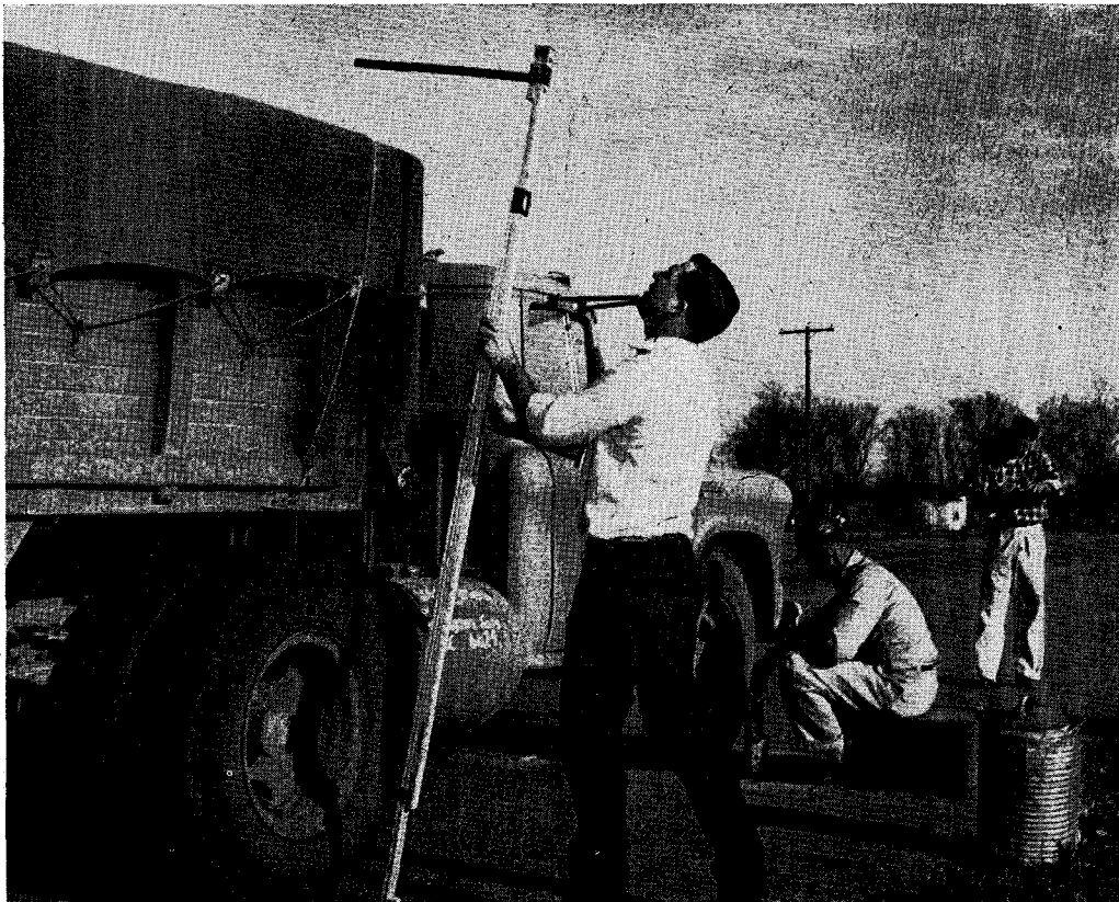
Figure 7 — Measuring height and front axle load, and identifying the vehicle.
