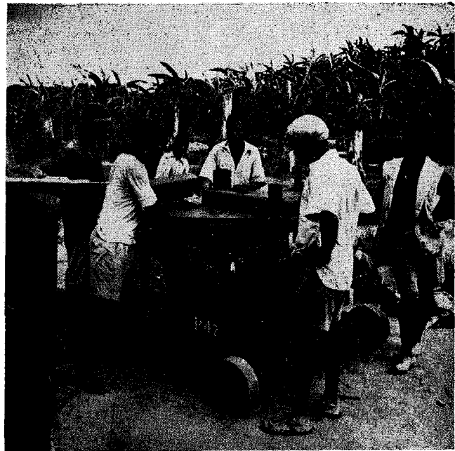
Figure 35. This Winget rotary block-making machine is being used in the British Cameroons.
