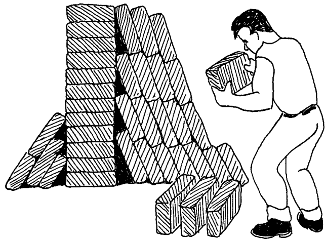
b. Cured block is stacked after three weeks.
