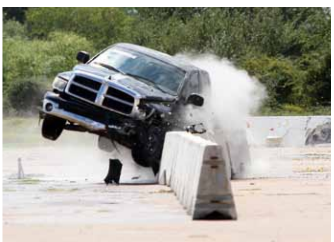
Homeland-security anti-terrorist, anti-ram structures and roadside safety devices are tested for durability at TTI's Proving Grounds Research Facility in Bryan.
