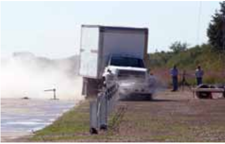
High-tension cable rail
