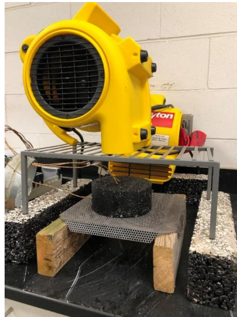
Figure 16. Rapid Cooling Unit with Two Fans.
