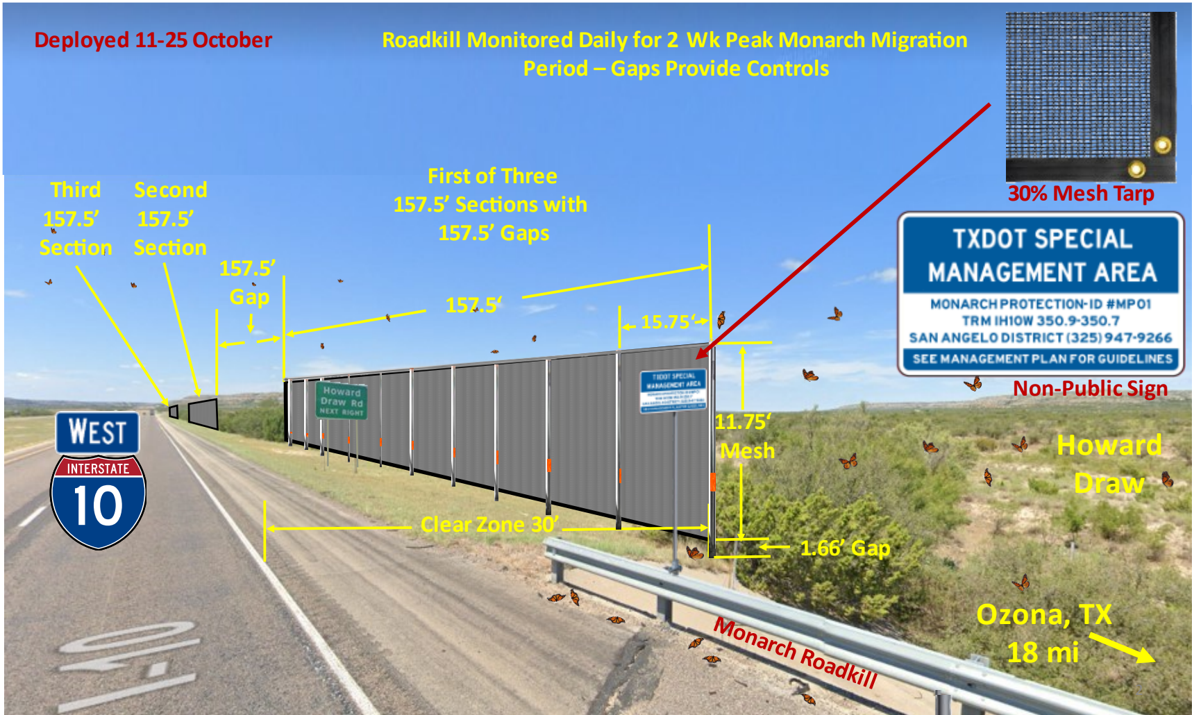
Figure 8.3. Design concept for land-based installation of three 157.5 ft sections of 12 ft height flight diversion mesh tarp at Howard Draw Specialized Management Area #MP01.
