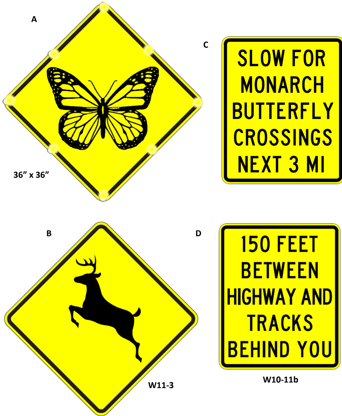
Figure D.2. Sign designs for (A) monarch crossing blinkersign; (B) deer crossing warning sign (W11-3) (TxDOT 2014c); (C) supplemental warning distance plaque with advisory non-specific speed reduction; and (D) warning storage space sign (W10-11b) (TxDOT 2014c).
