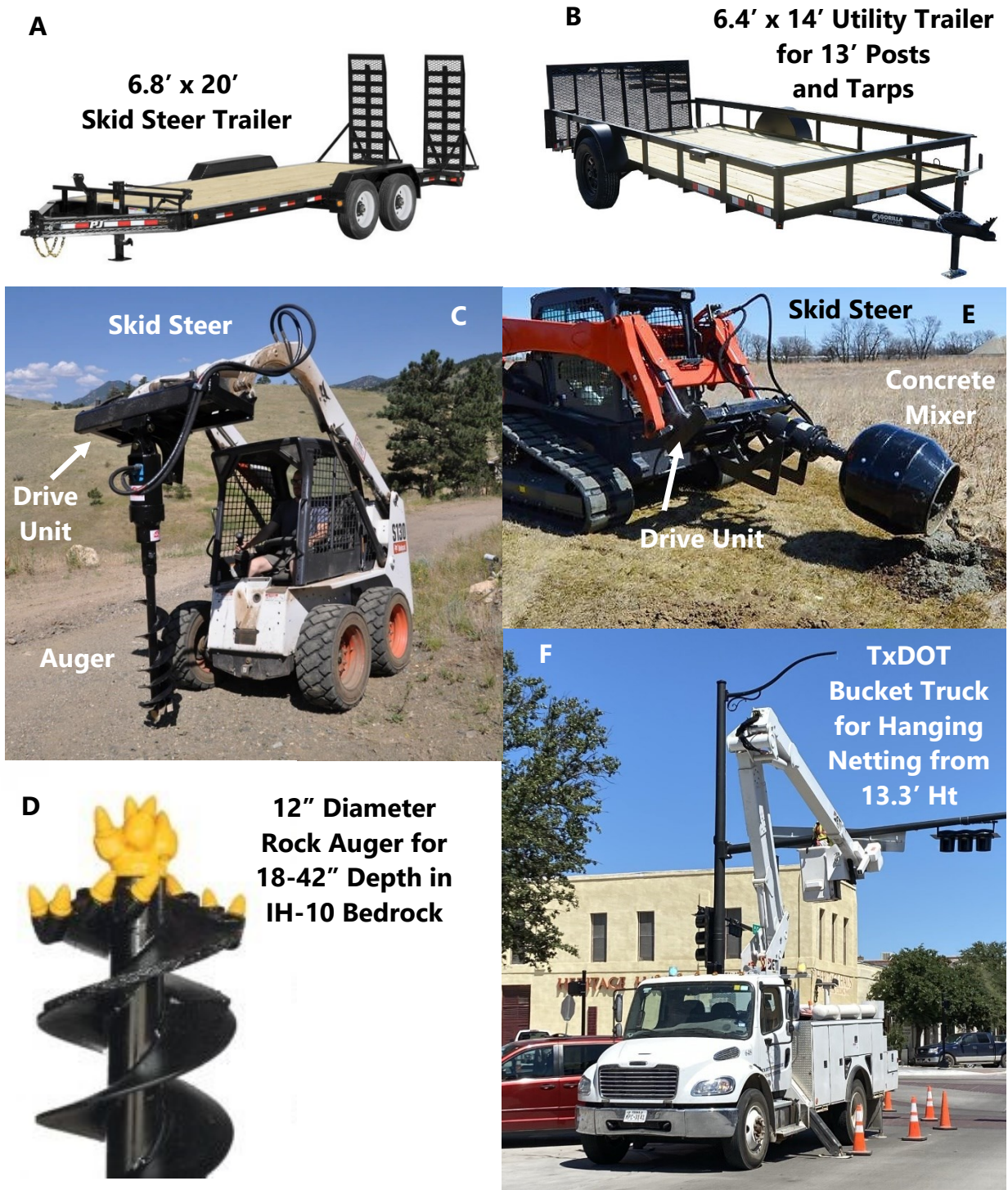
Figure 8.14. Heavy equipment for installation of flight diverter fencing installation along rocky roadsides.
