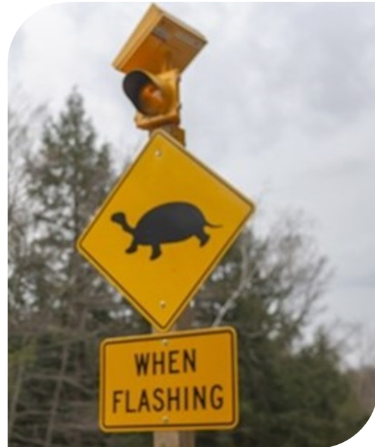
Figure 4.5. Turtle crossing temporal wildlife warning sign with flashing beacon in Aurora, Canada (Seyidova 2019)
