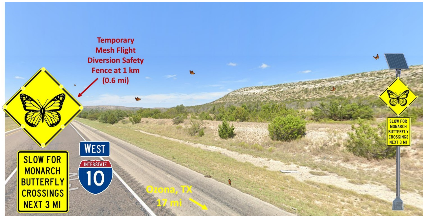
Fig. D.1. Design concept for land-based installation of monarch crossing blinkersign with supplemental warning non-specific advisory speed reduction at Howard Draw Specialized Management Area #MP01.
