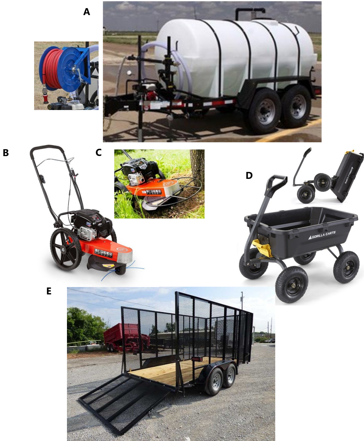
Figure 9.13. Equipment useful for installing and maintaining TxDOT pollinator habitat Specialized Management Areas: (A) 1000 gallon water buffalo tank trailer with hose attachment; (B) heavy duty trimmer mower with (C) vegetation/tree guard attachment, (D) seven cubic ft heavy duty poly yard dump cart for moving mulch and plants, and (E) 14' x 6.4' tandem axel straight utility cage trailer with mesh 6' sides for transporting mulch, cardboard, cart, and trimmer/mower.
