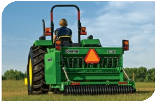
Figure 6.12. Frontier Conservation Seeder for tilling and seeding a wildflower meadow (JohnDeere.com 2019)
