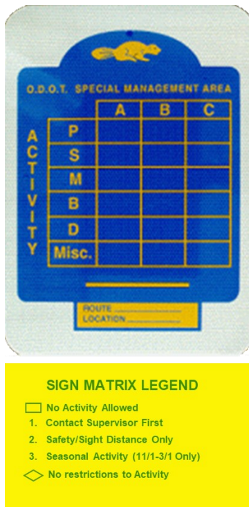
Figure 7.8. Oregon DOT Special Management Area coded instructions matrix sign (codes for activity to left and season codes across top) with yellow decoder card (AASHTO 2004).
