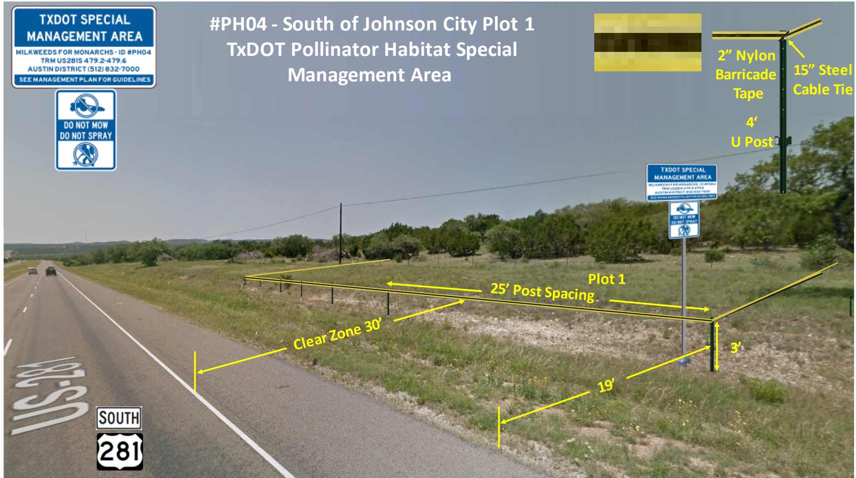
Fig. 9.6. Design concept for pollinator habitat Specialized Management Area (SMA) #PH04 with non-public TxDOT SMA and do not mow/do not spray signage for plot 1 located south of Johnson City.
