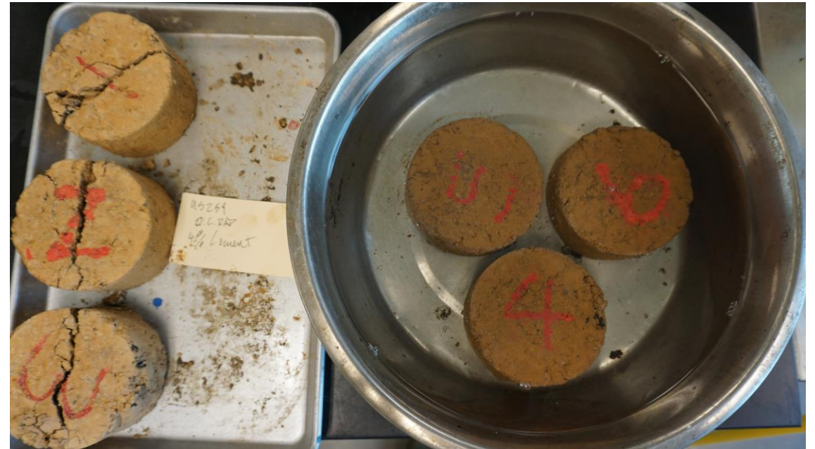
IDT Strength Specimens
