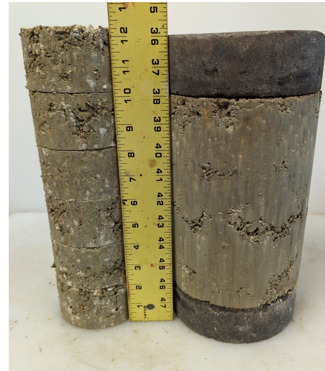
6 IDT Strength Specimens vs. 1 UCS Specimen
