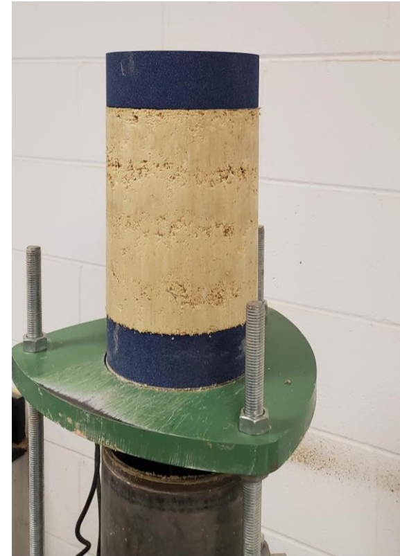
Example M-D Curve Specimen after Compaction
