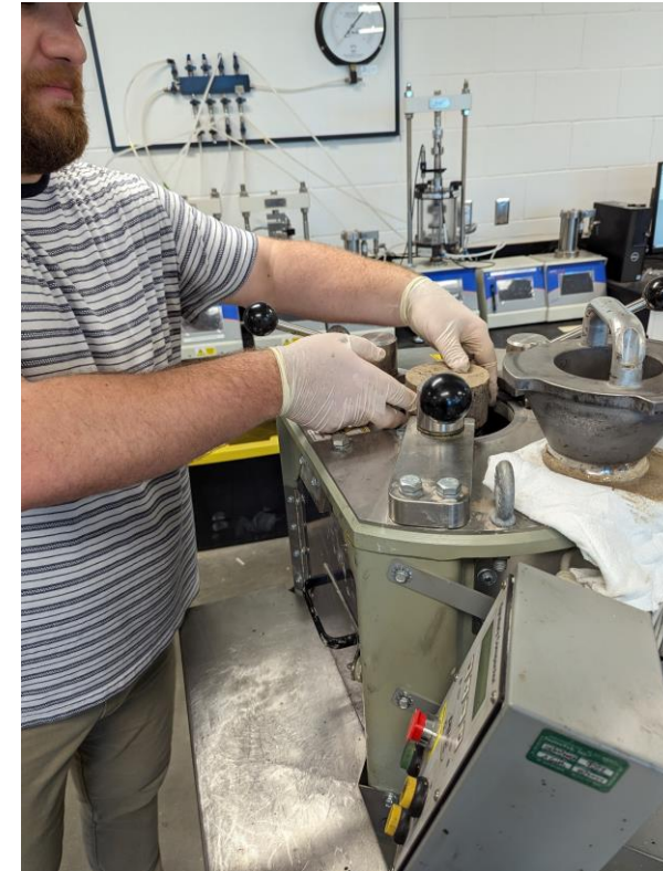
Extruding a 4×2 IDT Strength Test Specimen
