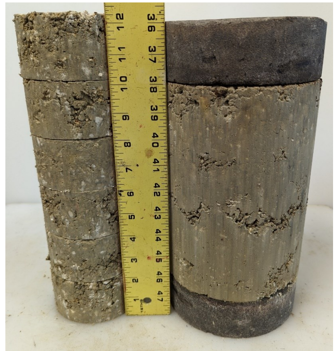
Figure 1. Rapid Mix Design Specimens (Left) versus Single Compressive Strength Specimen (Right) for CTB Mixture Design.
