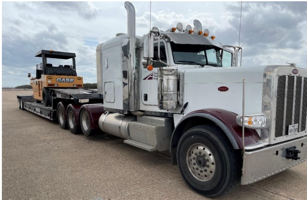
Figure 5.8. TTI Tractor-Trailer Loaded with a Roller Compactor.
