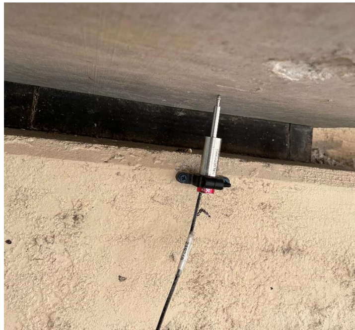
Figure 5.19. LVDT at South End (Bridge #2).
