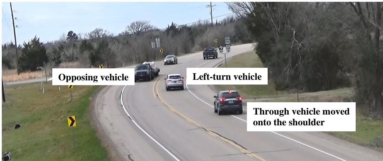
Figure 13. Vehicle Moved onto the Shoulder at the Study Site at SH 21 @ FM 1372.
