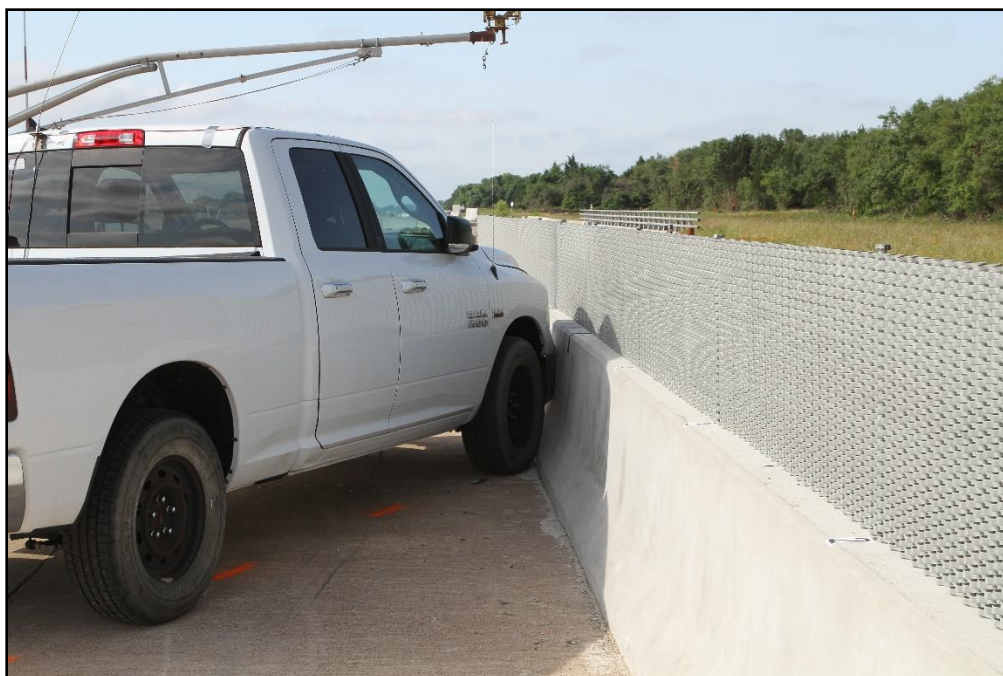
Figure 8.3. Screen-Safe® Glare Screen on F-Shape Barrier/Test Vehicle Impact Location, Test 440822-01-4.
