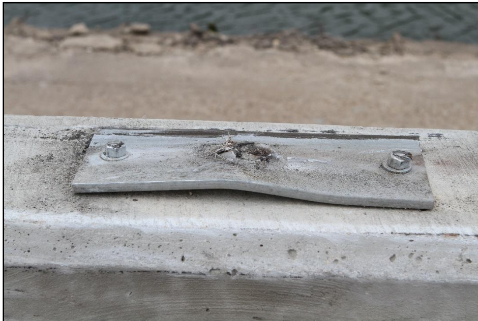
Figure 5.8. Armorcast® Gawk Screen on Single-Slope Barrier after Test at Base Plate with Missing Post, Test 440822-01-1.
