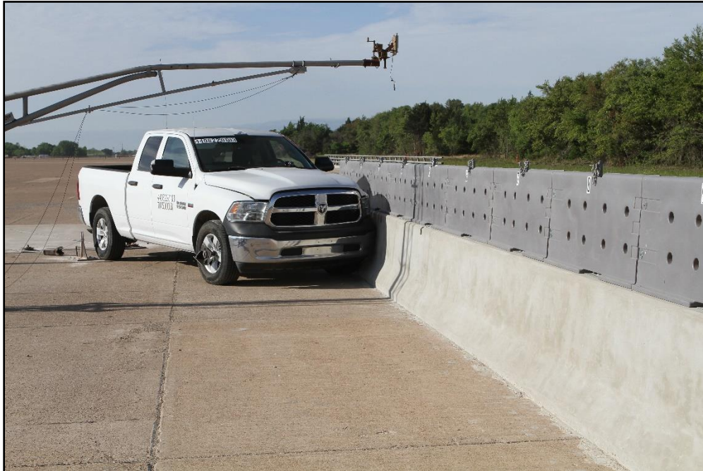
Figure 7.2. Armorcast® Gawk Screen on F-Shape Barrier/Test Vehicle Geometries for Test 440822-01-3.
