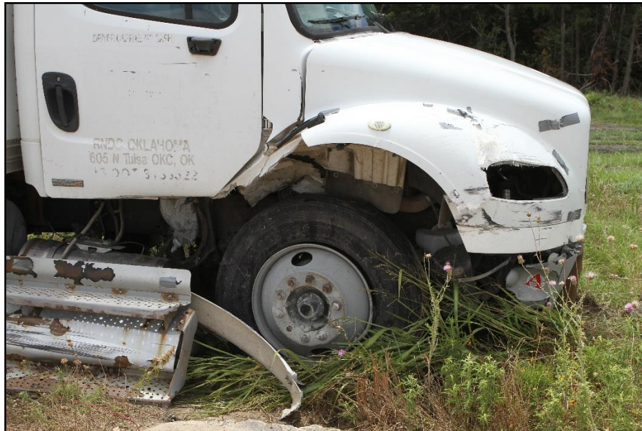
Figure 6.8. Impact Side of Test Vehicle after Test 440822-01-2.
