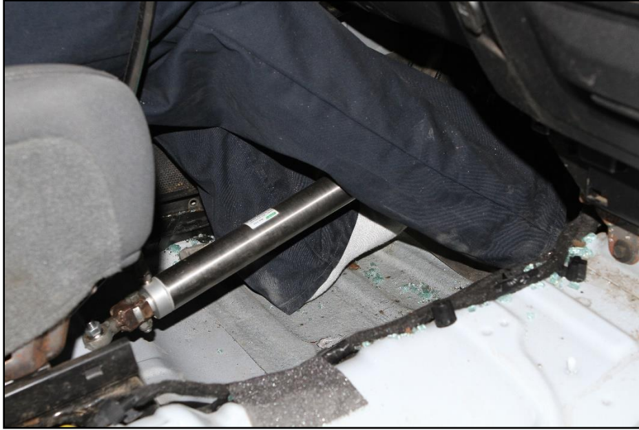
Figure 7.11. Interior of Test Vehicle on Impact Side after Test 440822-01-3.
