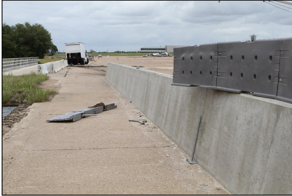
Figure 5.7. Rear View of the Armorcast® Gawk Screen on Single-Slope Barrier Post Impact, Test 440822-01-1.
