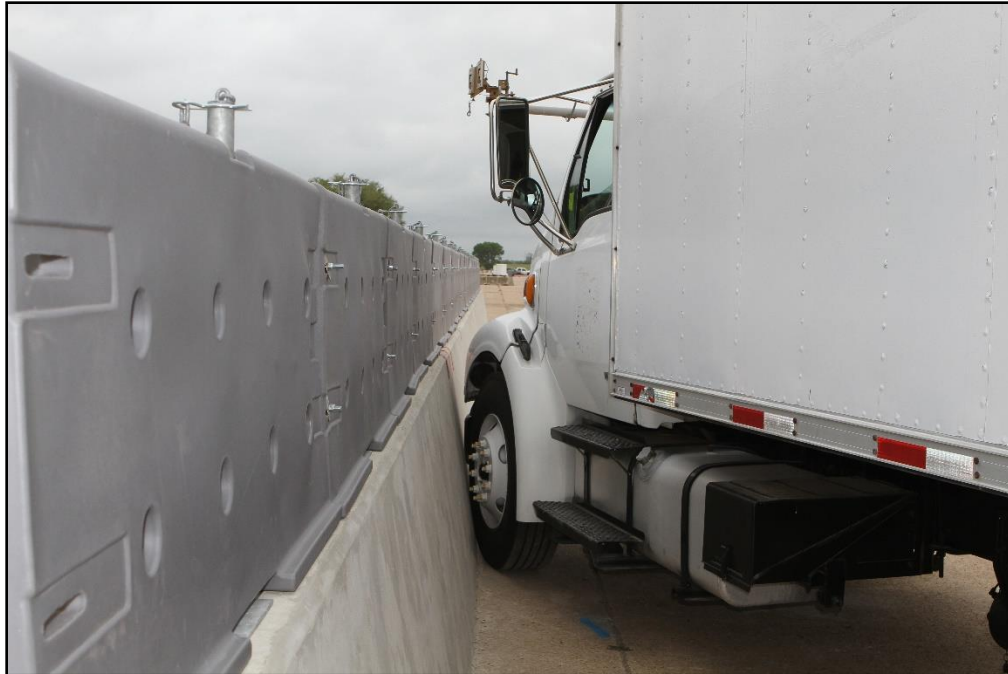
Figure 5.3. Armorcast® Gawk Screen on Single-Slope Barrier/Test Vehicle Impact Location for Test 440822-01-1.
