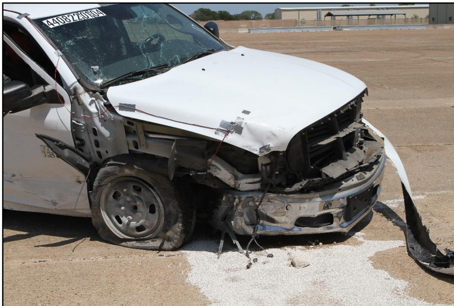
Figure 8.8. Impact Side of Test Vehicle after Test 440822-01-4.
