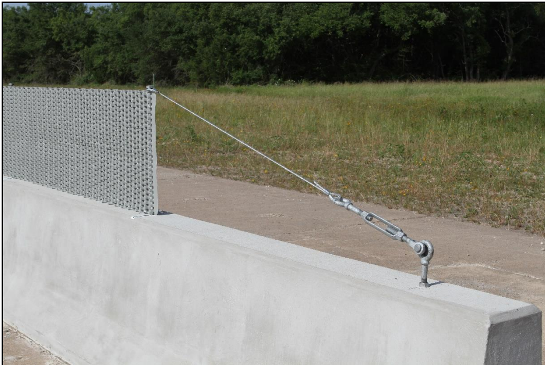
Figure 2.13. Screen-Safe® Glare Screen on F-Shape Barrier prior to Testing.
