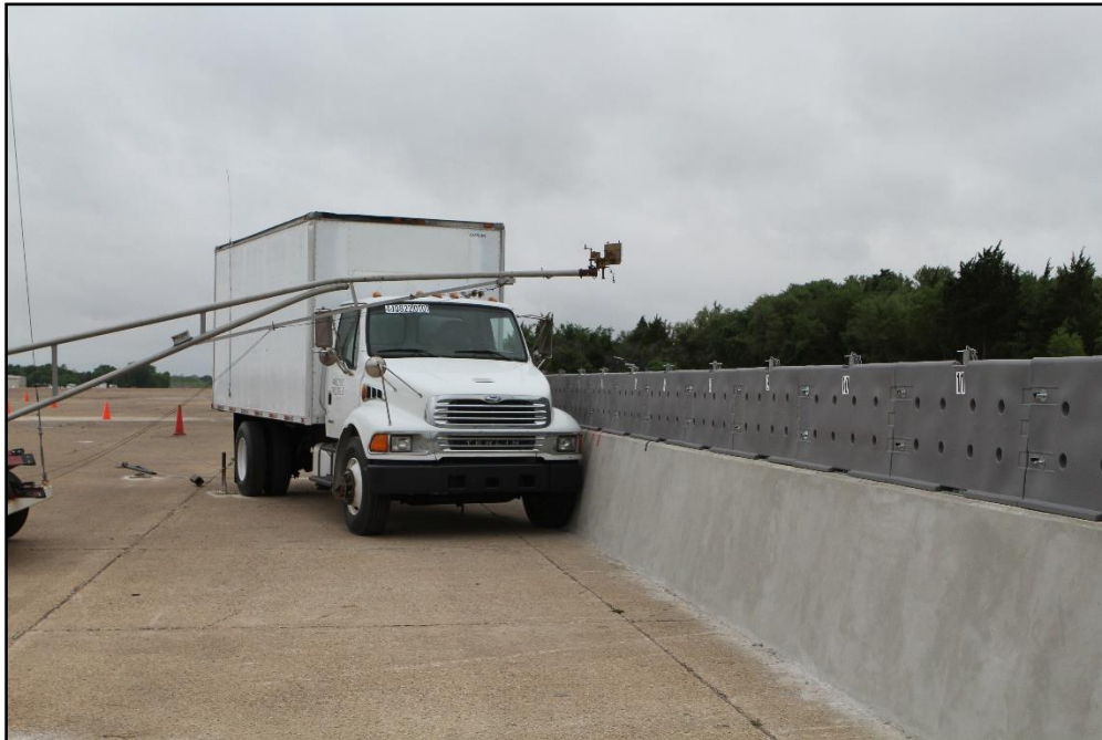
Figure 5.2. Armorcast® Gawk Screen on Single-Slope Barrier/Test Vehicle Geometries for Test 440822-01-1.
