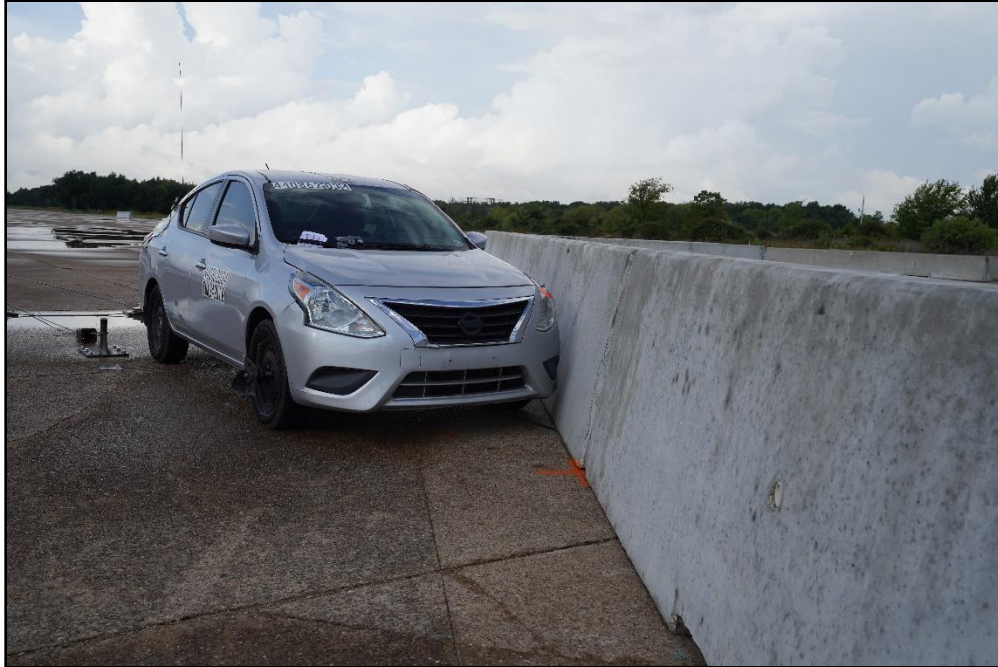
Figure 7.1. Flared Single-Slope Portable Concrete Barriers/Test Vehicle Geometries for Test 440862-03-4.
