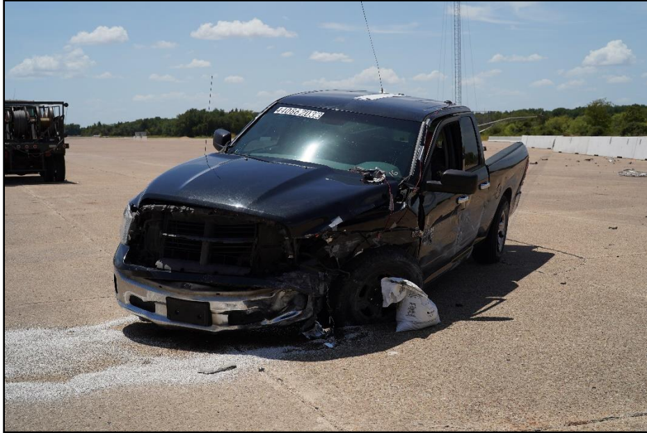
Figure 6.7. Impact Side of Test Vehicle after Test 440862-03-3.
