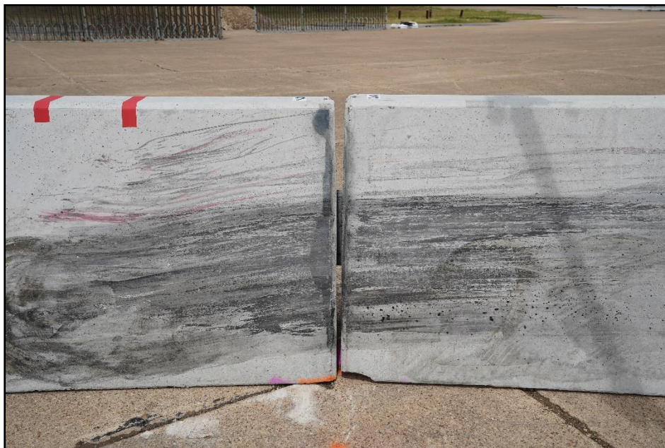
Figure 7.6. Flared Single-Slope Portable Concrete Barriers after Test at the Joint of Barriers 2 and 3, Test 440862-03-4.
