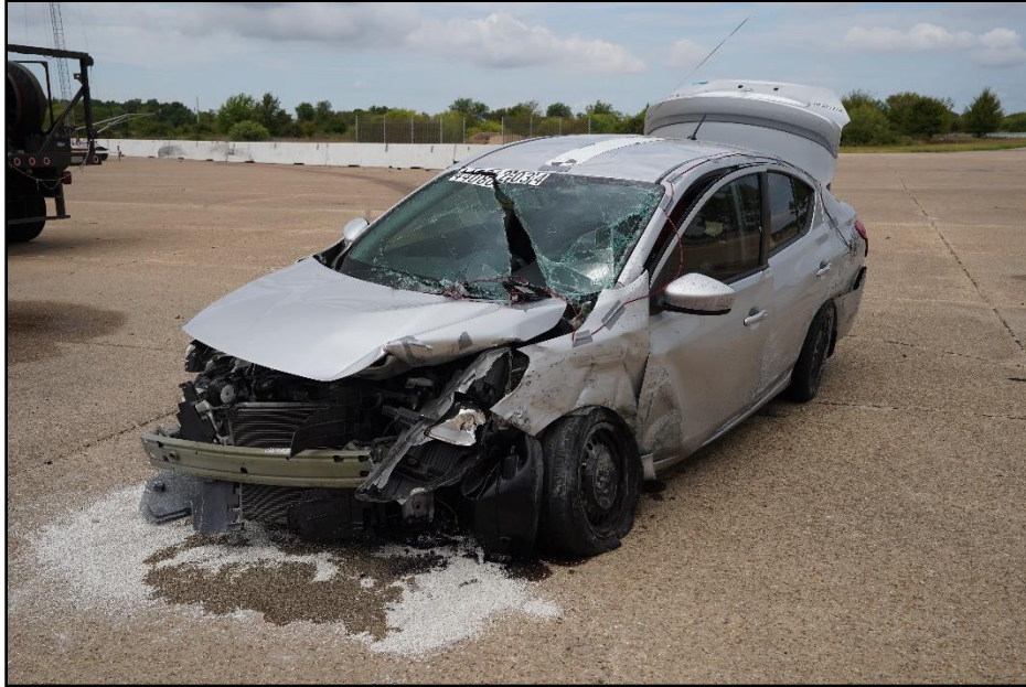
Figure 7.7. Impact Side of Test Vehicle after Test 440862-03-4.
