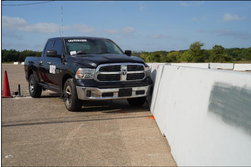
Figure 6.1. Flared Single-Slope Portable Concrete Barriers/Test Vehicle Geometries for Test 440862-03-3.
