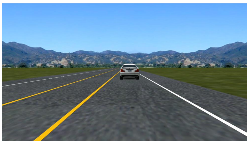
Figure 12. Experimental 8-ft Centerline Buffer Image—Treatment 5.
