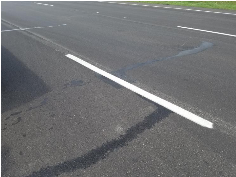
Figure 2. White Marking after Wet Retroreflectivity Evaluation.
