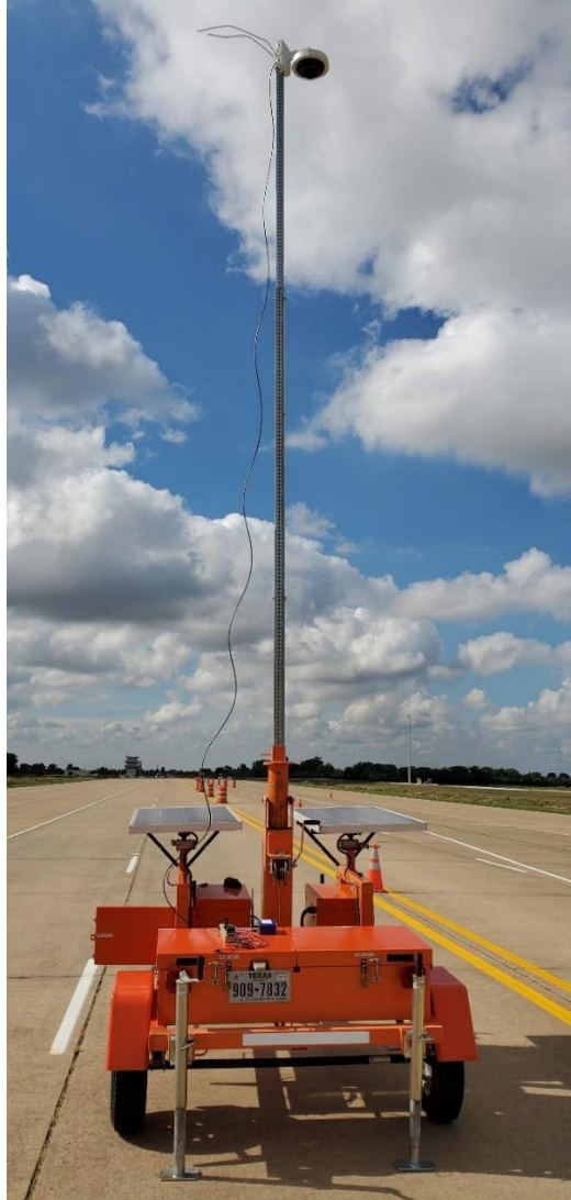
Figure 35. ISS Equipment on Portable Trailer.
