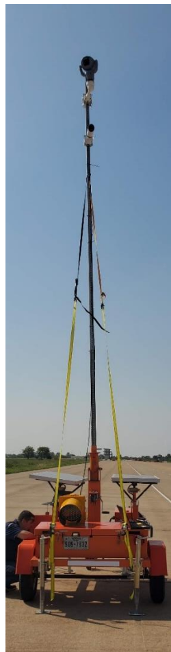
Figure 10. BOSCH Equipment on Portable Trailer.
