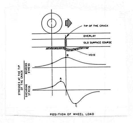
Figure 2.1. Stresses Induced at the Cracked Section Due to a Moving Wheel Load.
