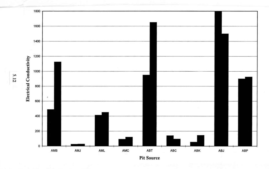
Figure 5.7 Ultimate Electrical Conductivity for Amarillo and Abilene Source Aggregates.
