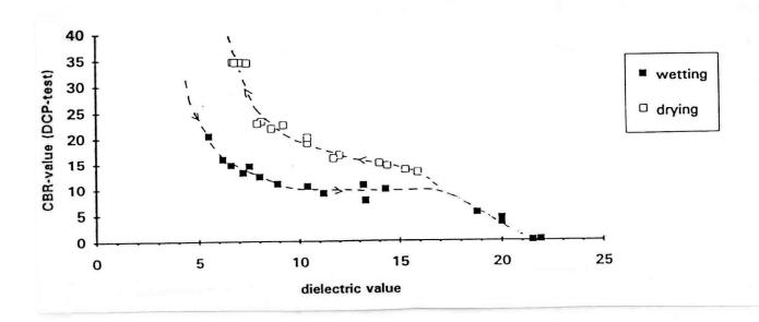
Figure 2.4. The Effect of Drying and Saturation in the Strength Properties and Dielectric Value of Some Texas Carbonate Aggregates.
