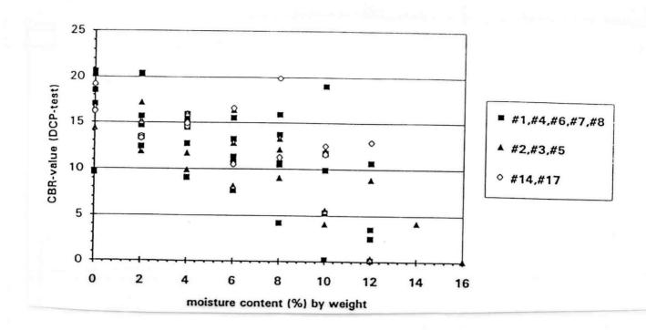
Figure 2.2. Correlation Between CBR-Value and Gravimetric Moisture Content of Texas and Finnish Aggregates.
