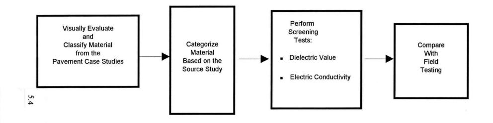
Figure 5.3 Flow Chart for Laboratory Testing of Pavement Case Studies.
