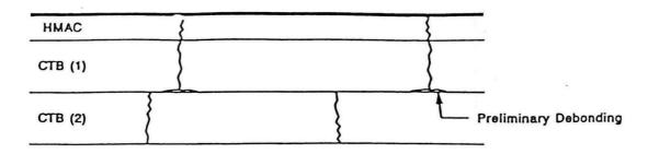
Phase 2 - Water ingress and deterioration under load.
