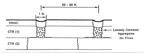
Figure 2.8. Deterioration Cycle of CRB on SH-36.
