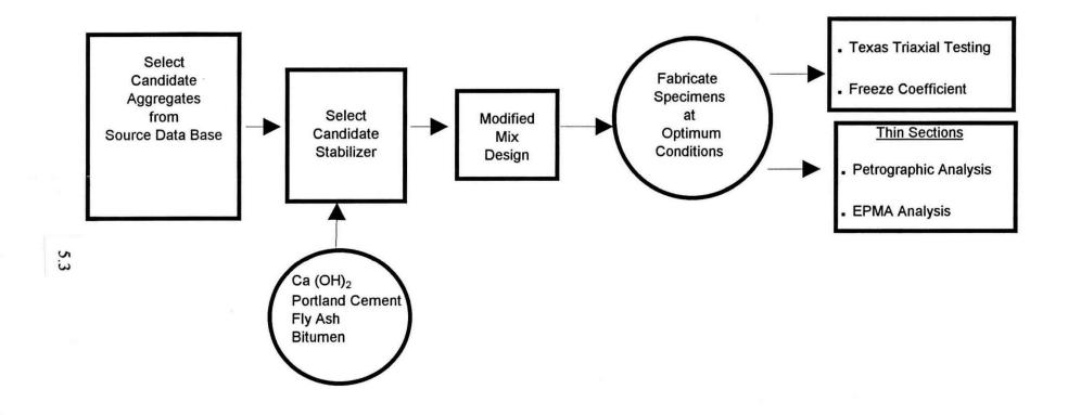
Figure 5.2 Laboratory Analysis of Stabilized Aggregate System.
