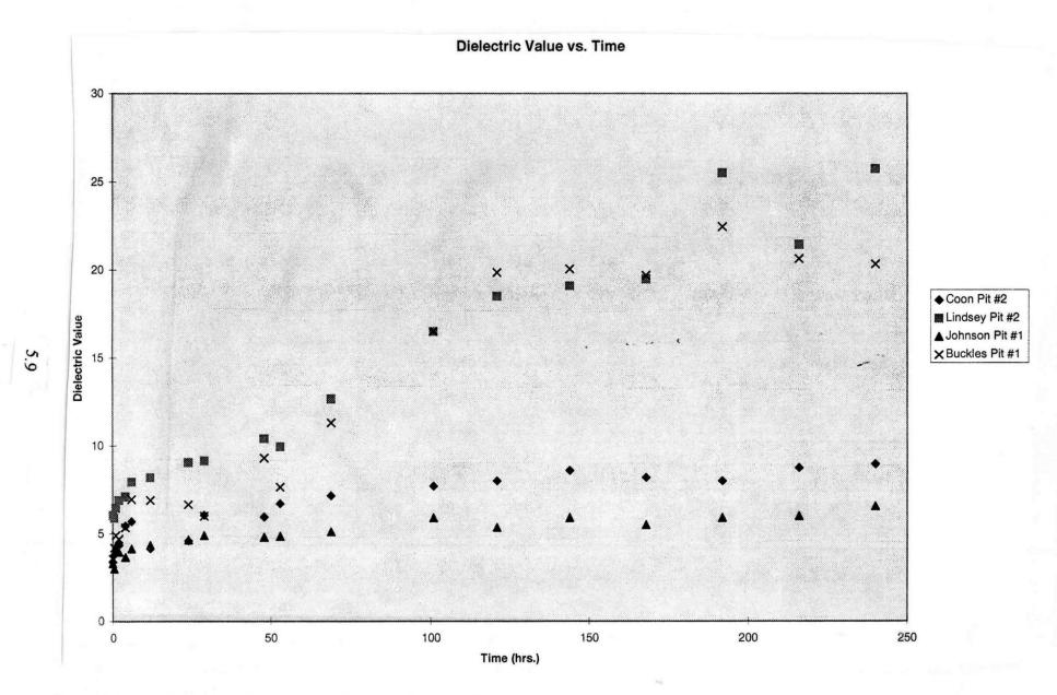
Figure 5.4 Dielectric Value v. Time of Testing for Amarillo Aggregates.
