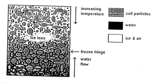
Figure 2.6. A Schematic Model of the Distribution of Water in Frozen Fringe.
