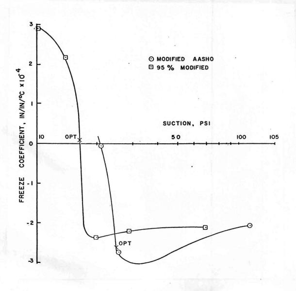
Figure 3.1 Freeze Coefficient as a Function of Suction for Material 4. After Carpenter and Lytton (1975).
