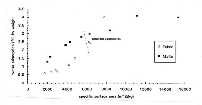
Figure 2.5. Correlation Between Water Absorption and Specific Surface Area of Fine Fractions (<0.074 mm) of Some Finnish Base Course Materials.
