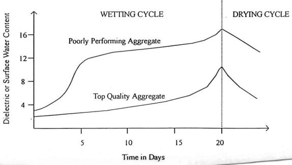
Figure 2.7. Schematic of the Suction Test and the Results of this Testing in Terms of Dielectric Constant Versus Time for Wetting and Drying Sequences.
