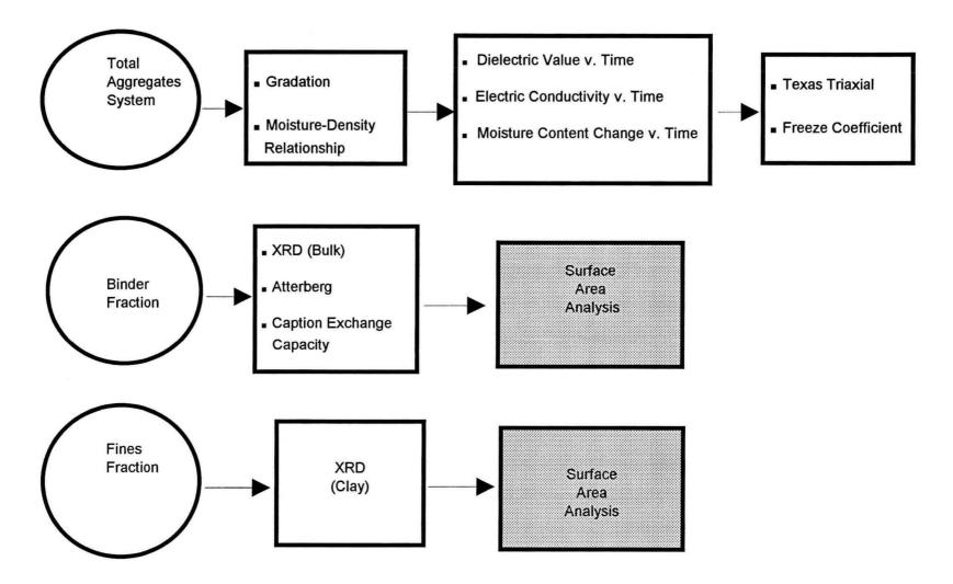
Figure 5.1 Laboratory Testing Sequence on Source Sample (From Amarillo District (4), Abilene (6), San Angelo (2) and Yoakum (2)).
