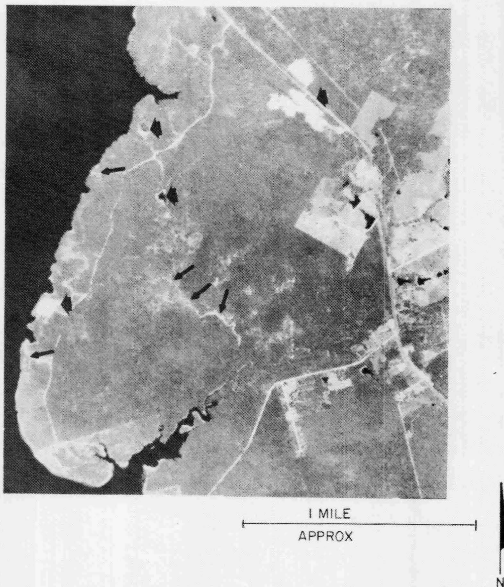
Figure 4. C-IR air photograph of sandstone prospect near Carlisle, Texas. Thin arrows point to light toned patches that represent near surface or outcropping sandstones. The thick arrows point to rock pits. (C-IR stands for Color-Infrared.)
