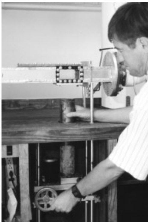
Dr. Jean-Louis Briaud operates the Erosion Function Apparatus, which tests the erodability of soil samples taken from the streambed.
