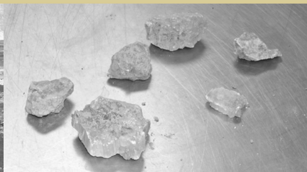
Left: Closeup of pavement heave. Soils underneath the surface can swell causing the pavement to heave. Right: Calcium deposits taken from a section of roadway in Laredo.
