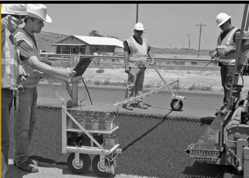
Left to Right: TxDOT's Steve Smith, TTI's Stephen Sebesta, TxDOT's Hector Flores and a member of the contractor crew use the first generation infrared imaging tool to test for segregation.
