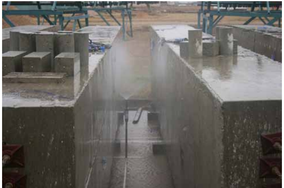
Concrete specimens are exposed to wetting and drying cycles by a sprinkler system at the TTI Riverside Campus to accelerate deterioration from ASR/DEF.
