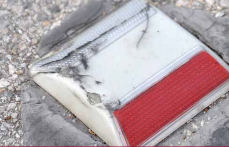
This pavement marker shows several failures on the shell. These failures could be caused by something as simple as a stone wedged in the tire tread of a vehicle.
