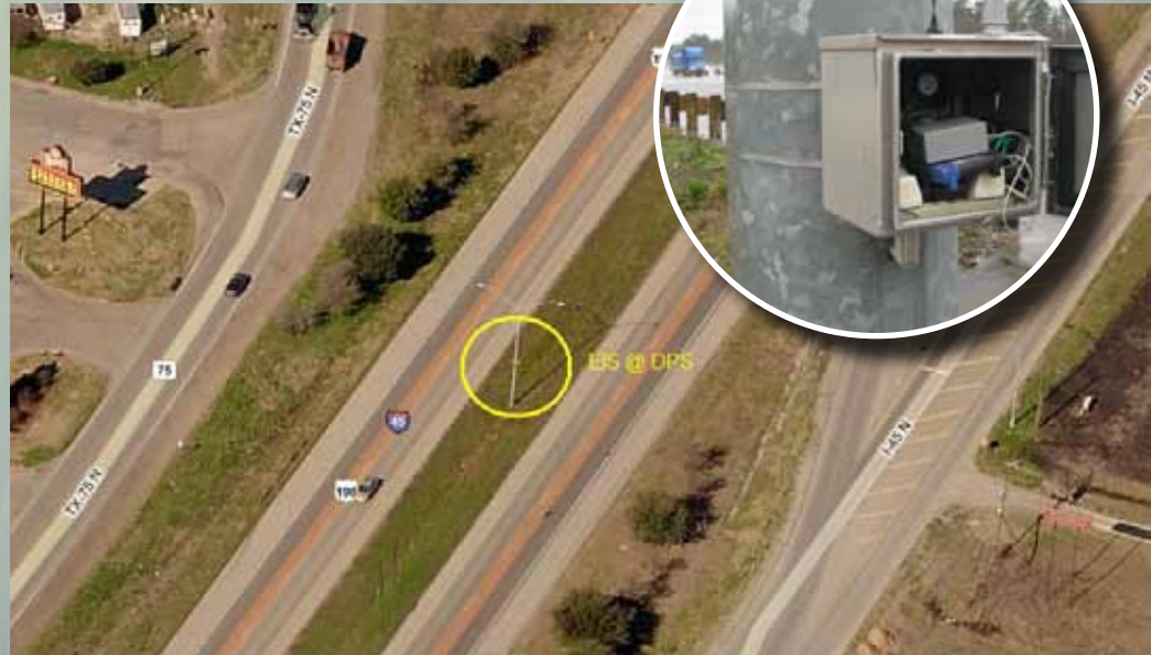
A bird's-eye view of a typical rural travel-time monitoring installation mounted on a luminaire pole. The inset photo shows a close-up of the prototype monitoring equipment.
