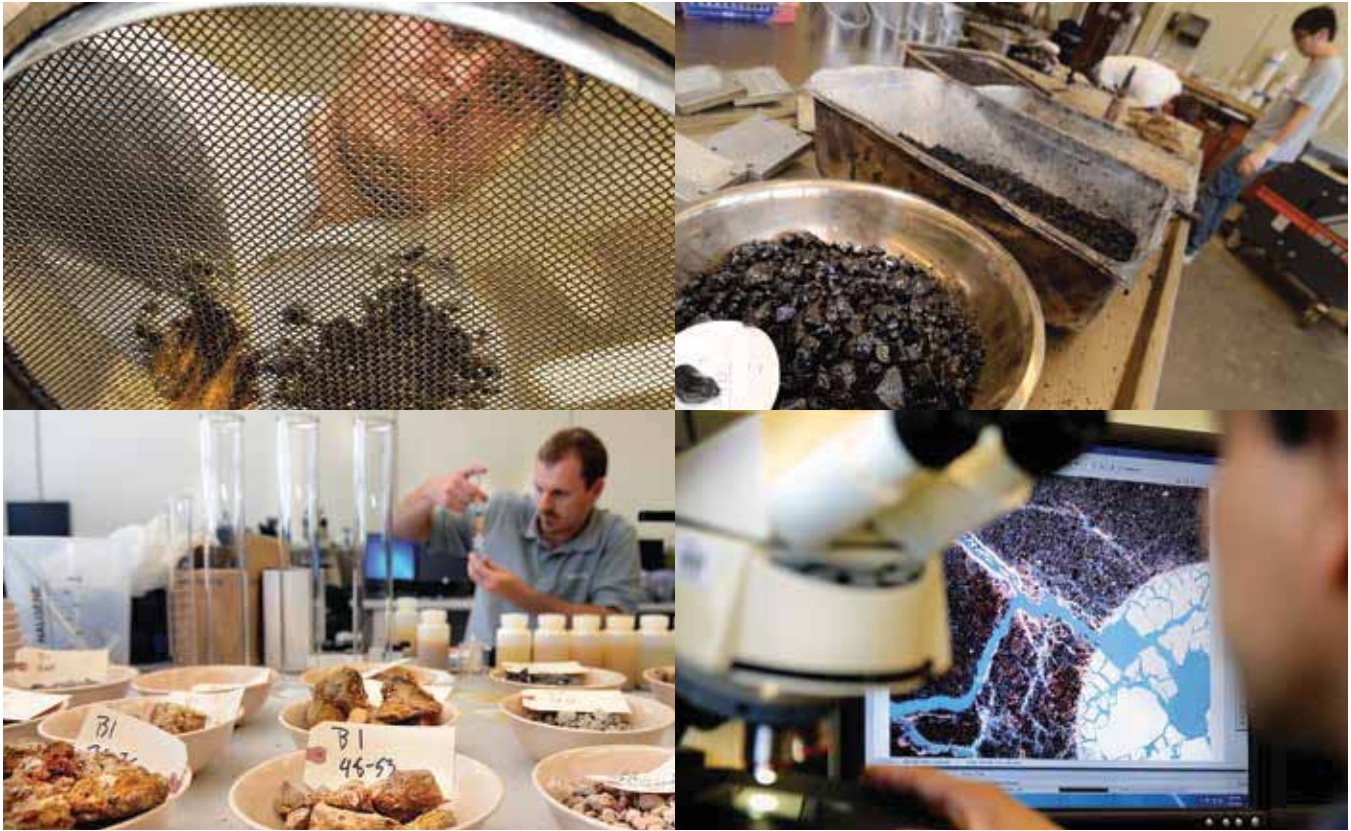
Top: Bulk materials processed in the McNew Lab become reconstituted to produce homogenous test specimens.
