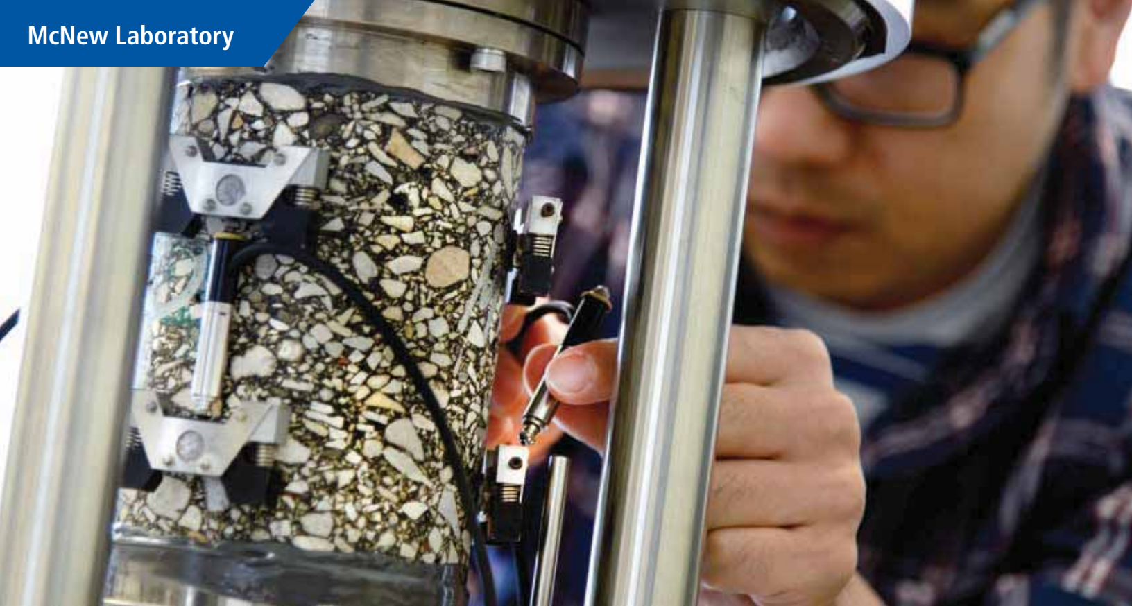
A TTI researcher instruments an asphalt specimen to measure its response under simulated traffic loading.
