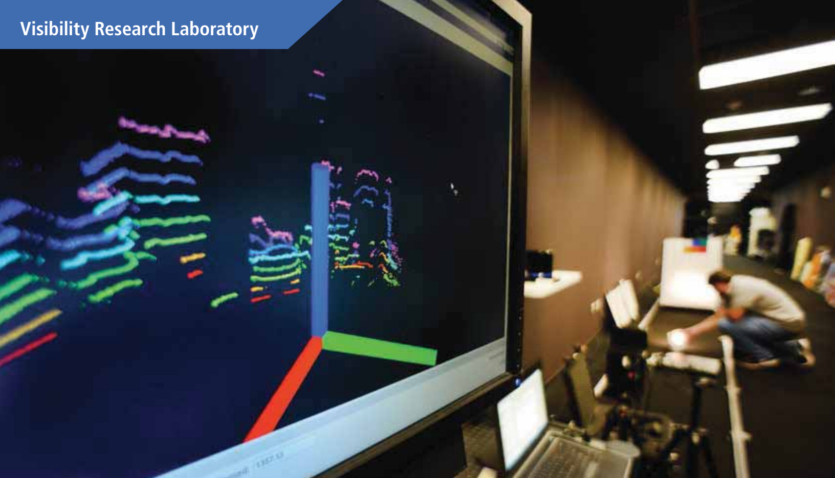
Evaluating the use of lasers to assess retroreflective infrastructure condition.
