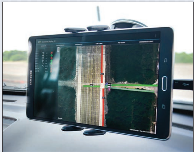
TTI has developed an augmented-reality environment where real entities (e.g., vehicles and traffic signal operation) are combined with simulated traffic and displayed on a screen.
