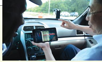
TTI researchers conducted an HITL simulation by integrating real CVs into a simulation model, simultaneously displaying simulated CVs inside the real vehicle.
