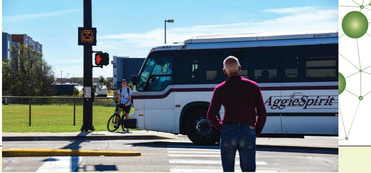
A Texas A&M University bus equipped with DSRC radios communicated its turn by activating the "Caution Bus Turning" warning and displaying a bus signal above the pedestrian sign. This Smart Intersection provides pedestrians, bicyclists and e-scooter riders a safer way to cross the street.
