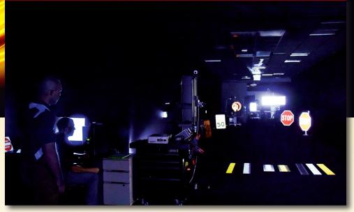
The lab has been used to measure the visibility of traffic control devices, retroreflective and luminescent materials, and light sources such as work zone lighting, light-emitting diodes and vehicle headlamps.
