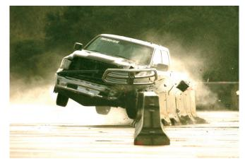
Roadside Safety and Hydraulic Drainage: TTI Proving Grounds researchers evaluate a concrete barrier with drainage structures with an impacting 5,000-pound pickup.
