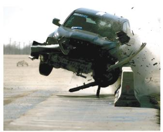
5,000-pound pickup truck impacts asphalt-pavement-mounted concrete barrier at 62 miles per hour.
