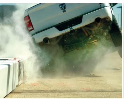
Low-profile barrier provides vehicular protection in work zones.
