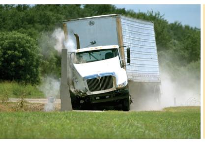
Noise abatement and roadway departure mitigation: 80,000-pound tractor-trailer contained by concrete barrier and soundwall.
