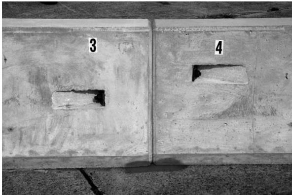
With TxDOT sponsorship, TTI developed a new, portable concrete barrier with an innovative connection that has the lowest deflection of any portable barrier in the country. And rather than waiting to schedule a crane to move standard, 30-foot barriers into place, the 10-foot lengths can be moved with a commonplace front-end loader—thus speeding up emergency responses and lessening the time it takes to deploy barriers on a job site. This development of a temporary concrete barrier
