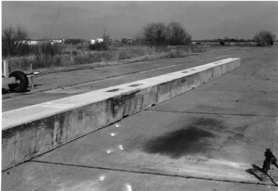
TTI developed a low profile portable concrete barrier that is designed for use at intersections in construction zones. This concrete barrier, about 12 inches shorter than the previous standard, allows drivers a greater field of vision. The barrier's shape is designed wider at the top to reduce the tendency for a vehicle to vault through the air on impact with the barrier.
