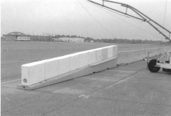
In the early 1990s, the Advanced Dynamic Impact Extension Module (ADIEM) barrier made of a soft crushable concrete called Perlite, also developed by TTI researchers, answered the demand for a cost-effective, easy-to-install crash cushion for concrete barriers. When struck by a vehicle, an ADIEM module absorbs the kinetic energy of the impact by disintegrating and slowing the vehicle to help bring it to a safe, controlled stop. FHWA acceptance for use on the NHS was granted on March 3, 1997.
