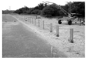
Despite designers providing wide medians between opposing traffic and improved high-speed roadway geometrics, motorists continue to cross over and have head-on collisions. The TTI researchers who were involved in crash testing both the low-tension and new generations of hightension wire rope cable barriers identified the need for a better performing terminal for high-tension longitudinal cable barriers.
