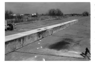
TTI developed a low profile portable concrete barrier that is designed for use at intersections in construction zones. This concrete barrier, about12 inches shorter than the previous standard, allows drivers a greater field of vision. The barrier's shape is designed wider at the top to reduce the tendency for a vehicle to vault through the air on impact with the barrier.
