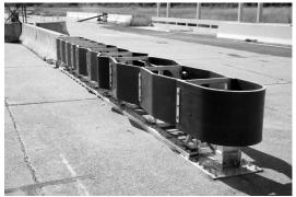
In the early 2000s, TTI researchers developed a crash cushion that can be reset and reused after being impacted. The goal was to develop a high performance crash cushion that had the potential to reduce maintenance costs to the states by potentially being re-useable after an impact. The result was a crash cushion fabricated from high-density-high molecular weight polyethylene (HDPE) plastic. Upon impact the flat HDPE side panels fold at predetermined hinge points and allow the crash
