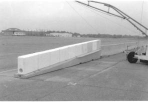
In the early 1990s, the Advanced Dynamic Impact Extension Module (ADIEM) barrier made of a soft crushable concrete called Perlite, also developed by TTI researchers, answered the demand for a cost-effective, easy-to-install crash cushion for concrete barriers. When struck by a vehicle, an ADIEM module absorbs the kinetic energy of the impact by disintegrating and slowing the vehicle to help bring it to a safe, controlled stop. FHWA acceptance for use on the NHS was granted on March 3, 1997.
